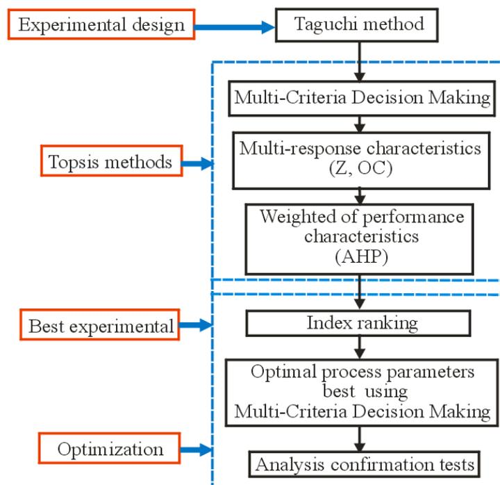
Fig. 2. Diagram of multi-criteria decision making using Taguchi – AHP- TOPSIS [27]
