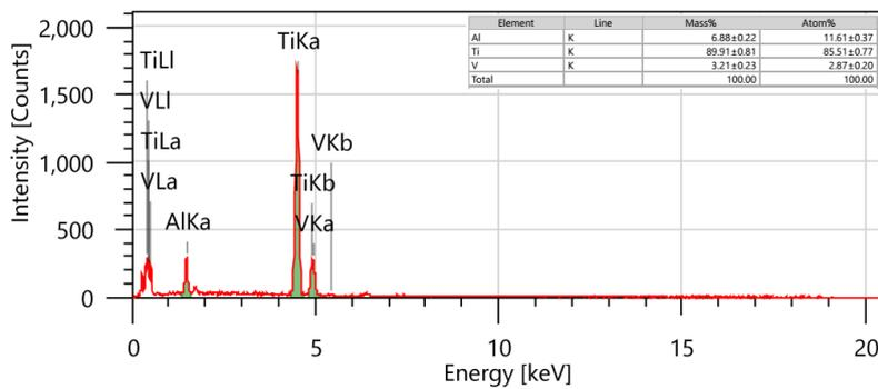
Figure 7. SEM- EDX of Ti-6Al-4V workpiece
