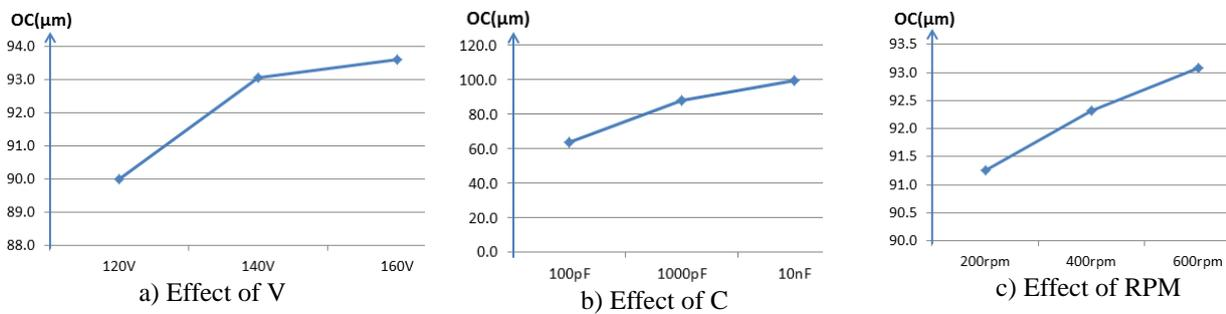
Fig. 4. Effect of V, C and RPM on OC
