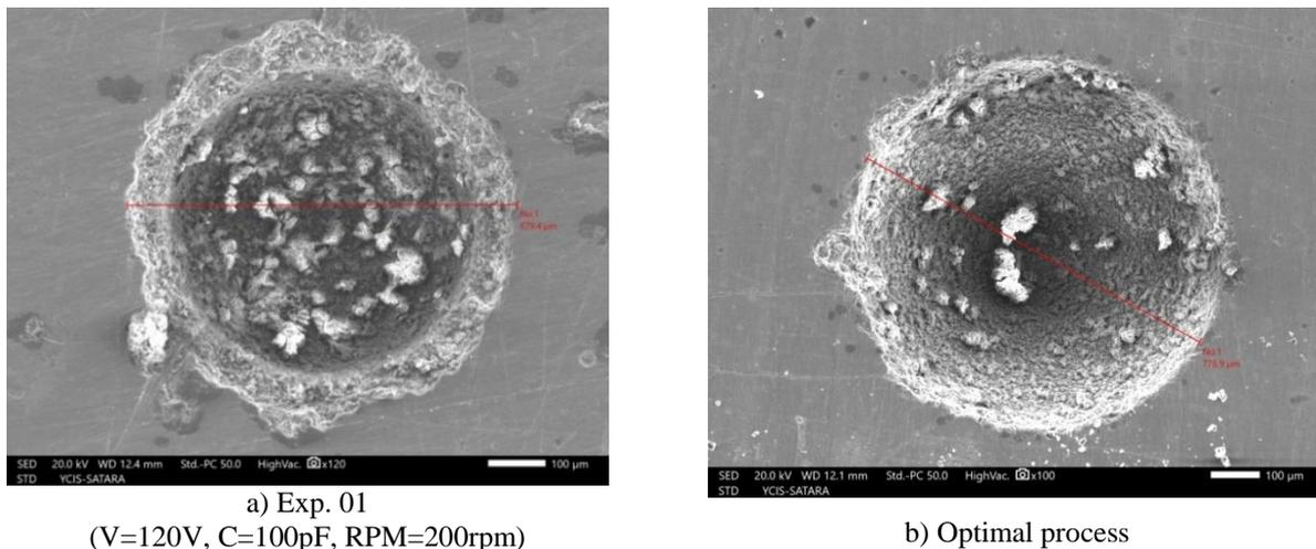
Fig. 5. SEM of micro- hole in  $\mu$ -EDM at optimization process
