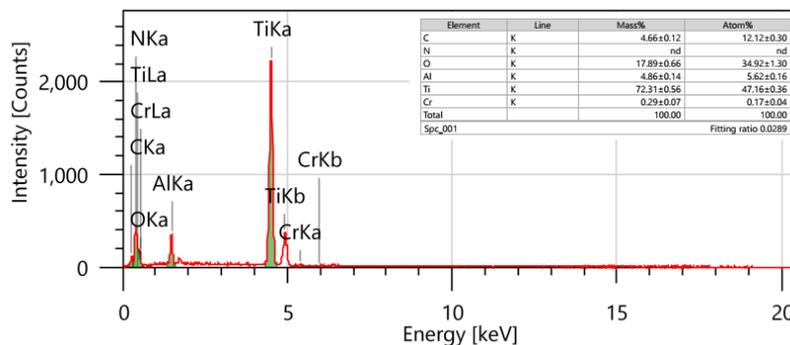
Fig. 8. SEM- EDX of machined surface after micro-EDM with WC electrode
