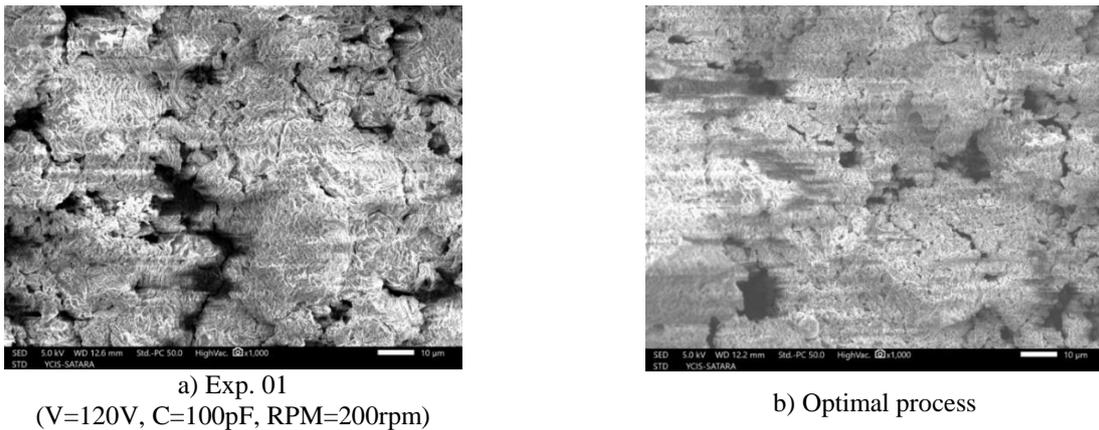
Fig. 6. Micro-cracks on machined surface in  $\mu$ -EDM
