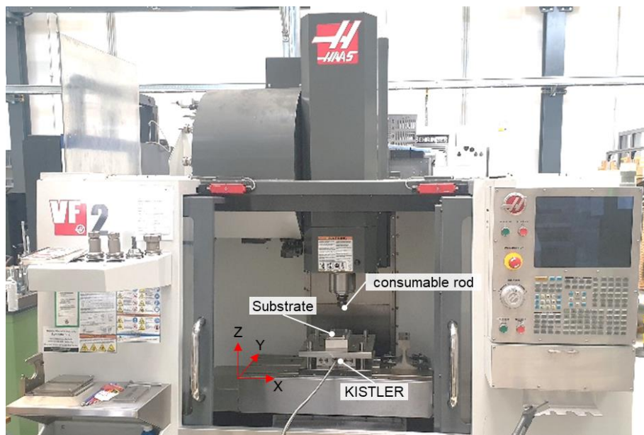
Fig. 2. Experimental setup for friction surfacing tests at TU Wien
