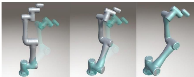
Fig. 4. DT and ghost robot when the position is published(left), midway(center), and having reached the goal state(right)
