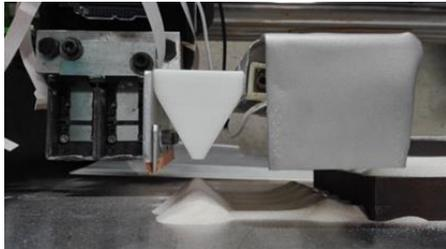
Fig. 23. Hopper mounted on the jig
