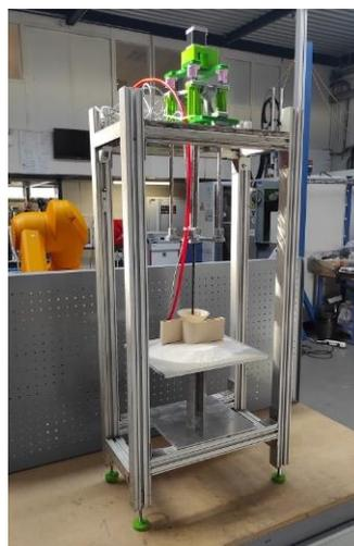
Fig. 14. A 200 mm diameter x 600 mm prototype 1 dof machine
