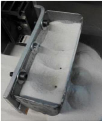
Fig. 17. Flow of sand stopped
