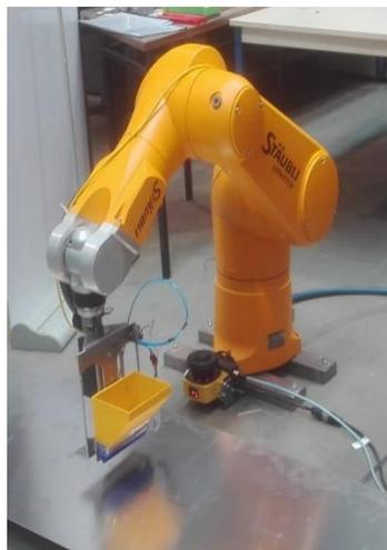
Fig. 4. Staubli TX90 6 axis robot with the sand deposition tool
