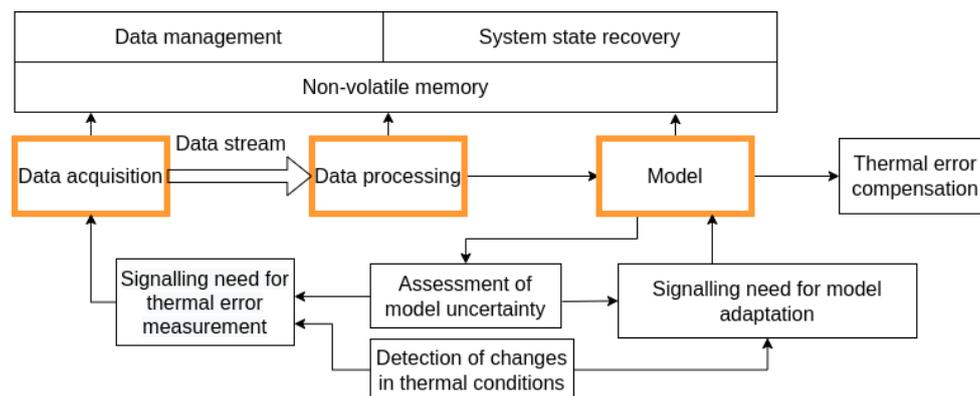
Fig. 2. Self-compensation system structure with highlighted main machine learning components
