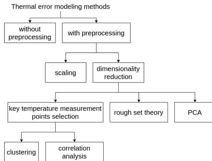
Fig. 4. Division of thermal error modelling methods with regard to data processing
