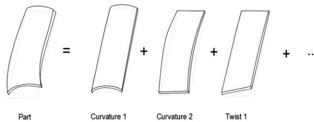
Fig. 15. Digital twin modeling as a combination of known features [19]
