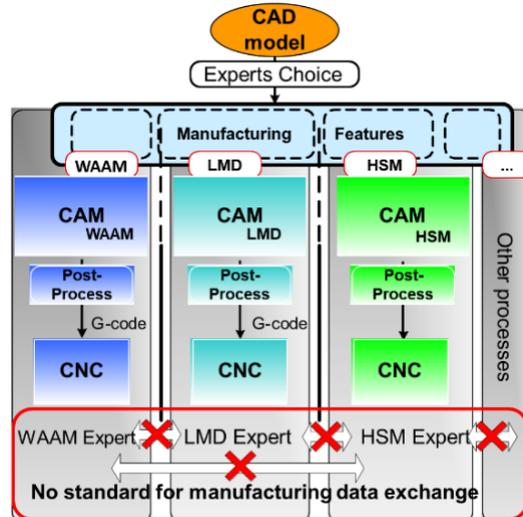
Fig. 3. Current numerical data chains for hybrid manufacturing
