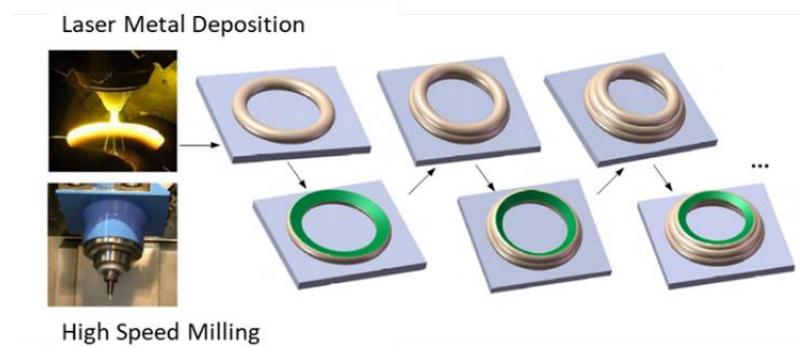
Fig. 2. Example of hybrid approach by sequentially combine additive and machining processes
