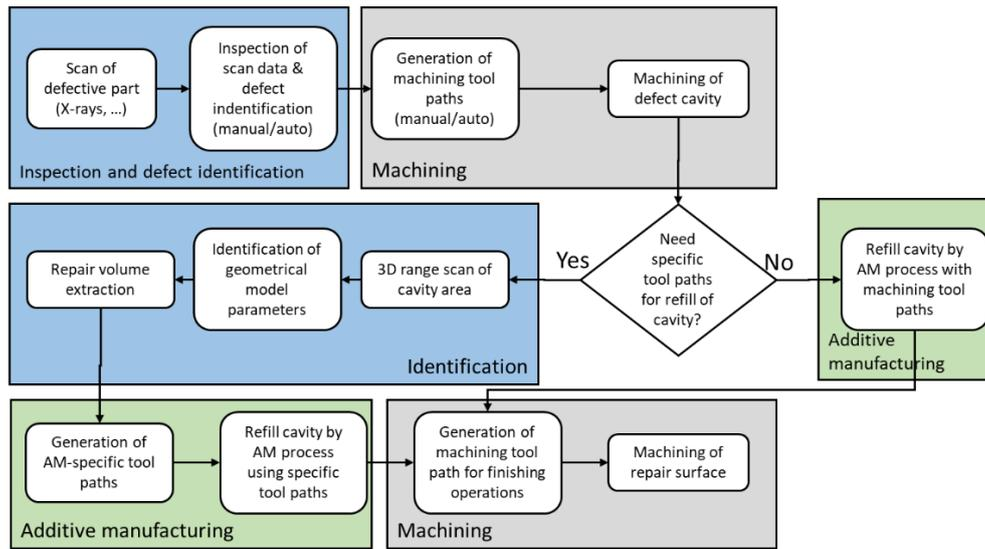
Fig. 6. Semi-automatic hybrid repair method
