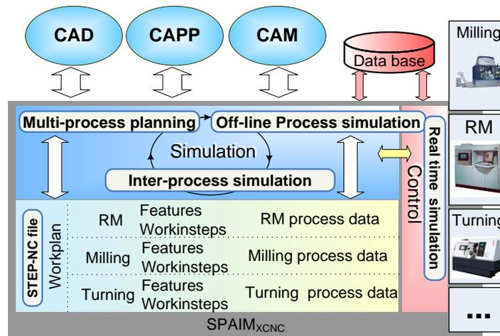
Fig. 11. Coupling offline simulation and STEP-NC controller for multiprocess manufacturing
