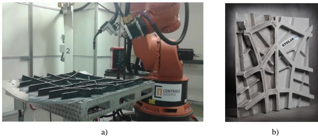
Fig. 9. Self stiffened panel: a) – during the additive manufacturing phase, b) – after machining and painting
