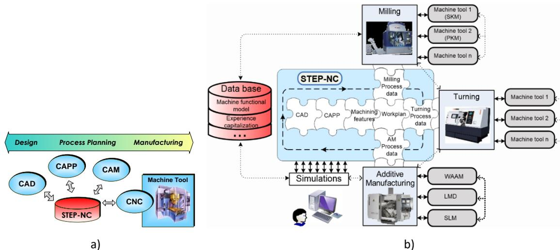
Fig. 4. STEP-NC approach: a) vision of numerical data chain, – b) multiprocess environments
