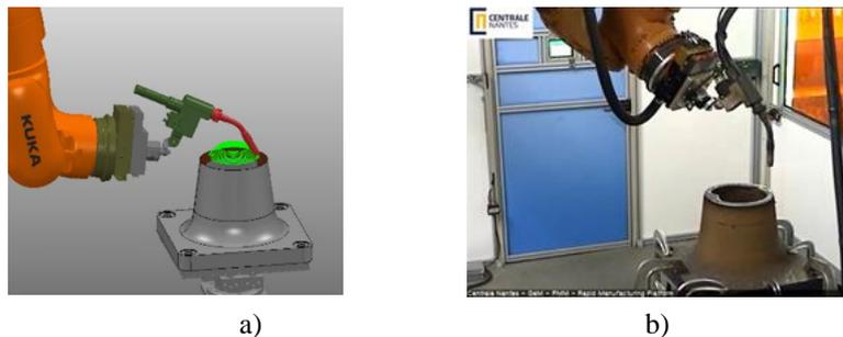
Fig. 13. Interest of the digital twin to generate complex tool paths: a) – tool path generation in the virtual environment with the digital twin, b) – tool path execution in the real environment
