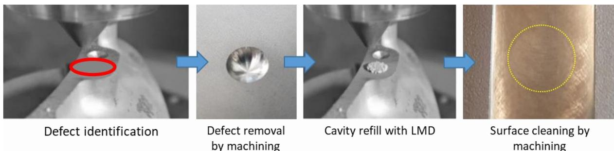
Fig. 7. Examples of aeronautical components repair with the proposed method
