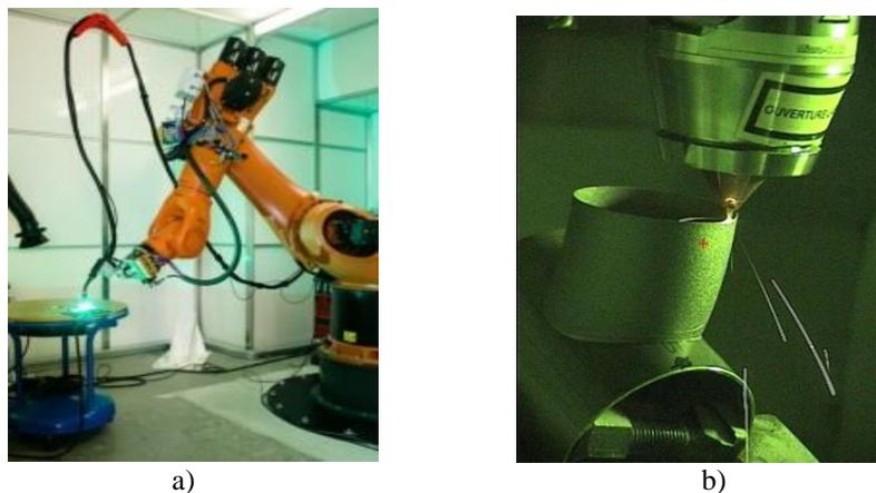
Fig. 1. Additive manufacturing processes: a) wire arc additive manufacturing – b) laser metal deposition
