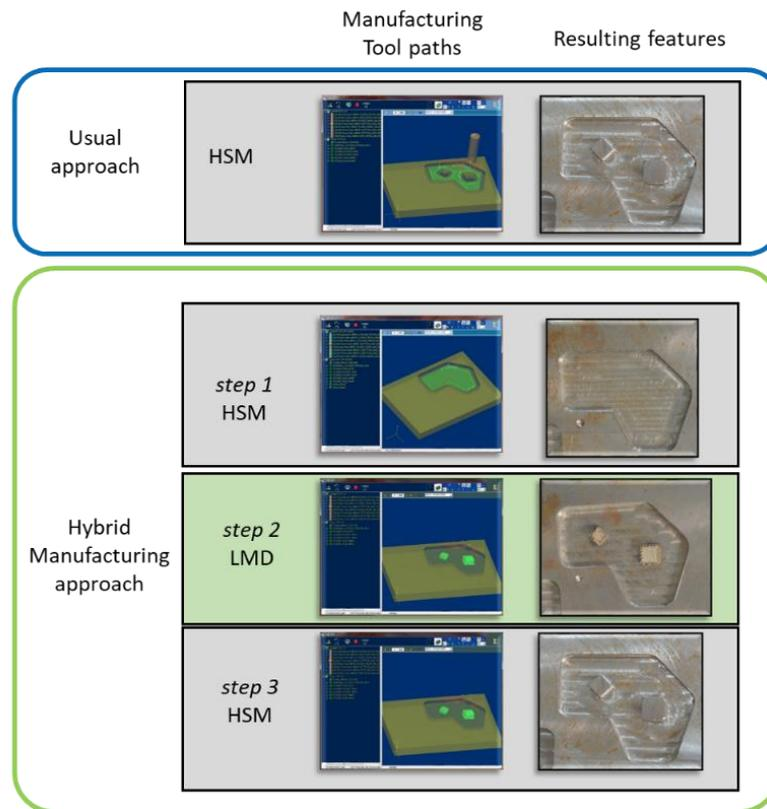
Fig. 5. Example of usual vs hybrid manufacturing approaches with STEP-NC
