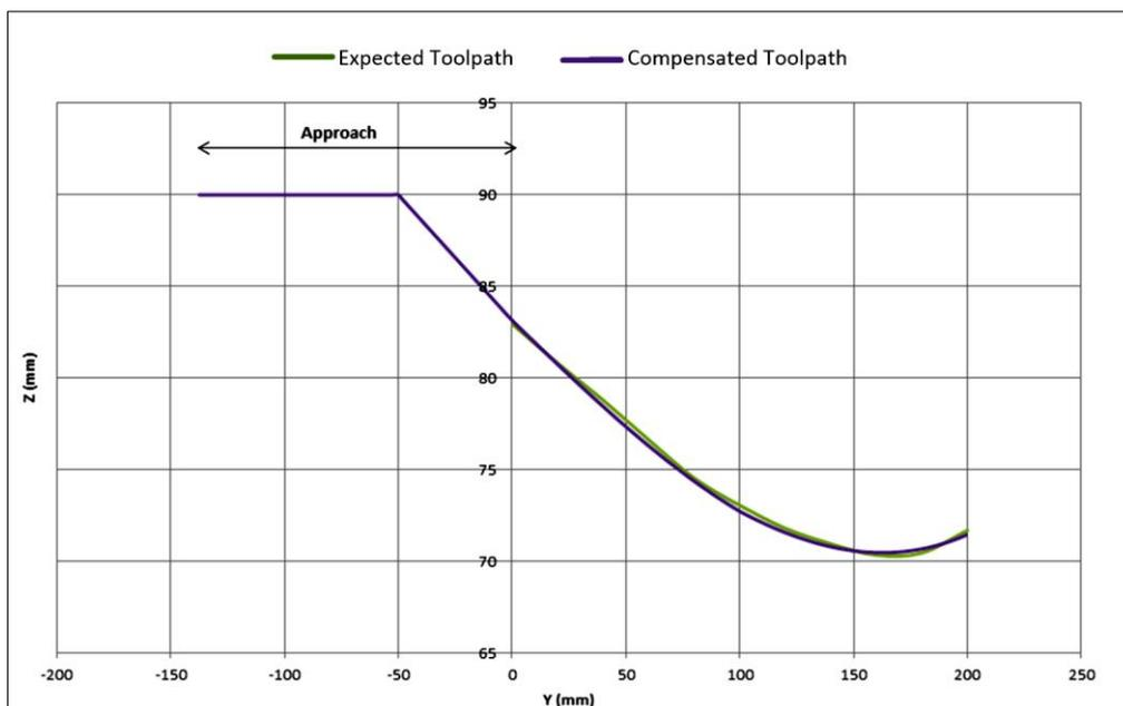
Fig. 16. Comparison of expected and compensated toolpaths for a curved sheet metal [3]
