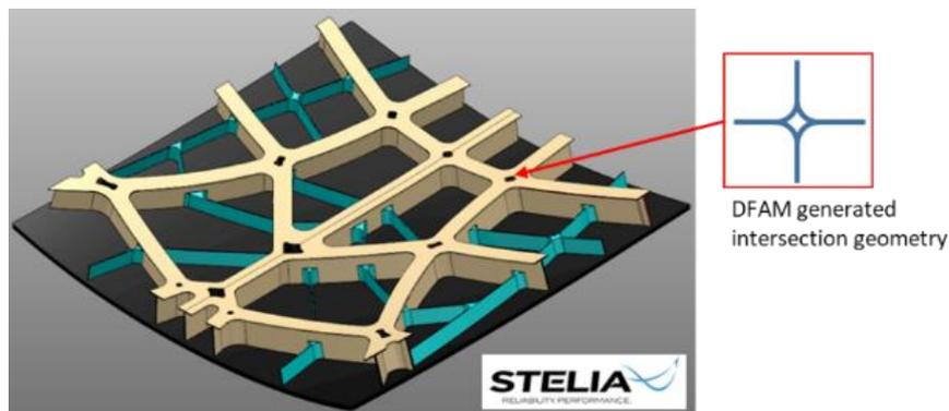
Fig. 8. Structural panel demonstrator after DFAM
