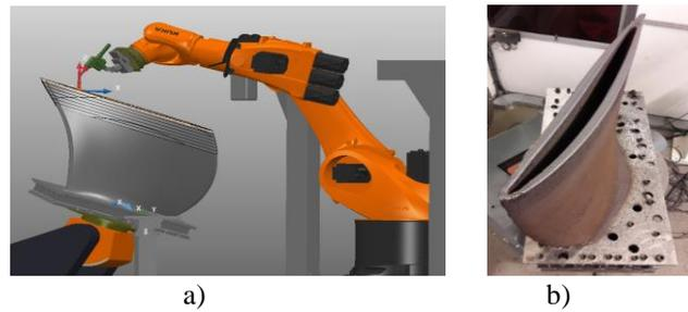
Fig. 12. a) – Control of the melting pool orientation by using the digital twin of the manufacturing cell, b) – View of the hollow blade during manufacturing
