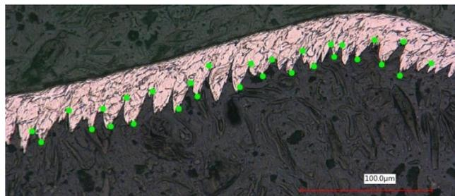
Fig. 21. Very irregular chip segmentations can cause problems in the automated extreme point determination, here on a chip generated at a very low feed rate of  $f = 0.01$  mm/rev (experiment V0001 from [12])
