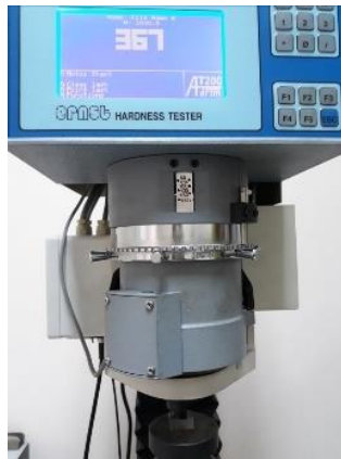
(a) The Brinell hardness at the experimental No. 12
