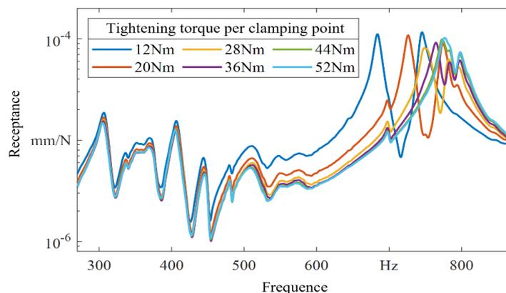
Fig. 8. Receptance for different tightening torques of the down-thrust clamp (excitation point 21/29, measuring point 28)
