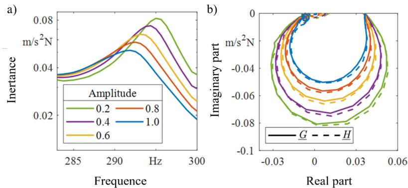
Fig. 7. Nonlinear measurement at 295 Hz: a) inertance for different excitation amplitudes in the Bode plot, b) comparison of the FRF ( $\underline{G}$ ) with its Hilbert transform ( $\underline{H}$ ) in the Nyquist plot
