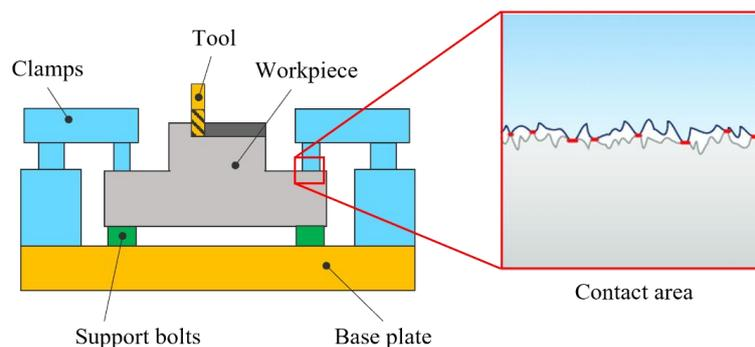
Fig. 1. Illustration of the contact area between the workpiece and clamping elements
