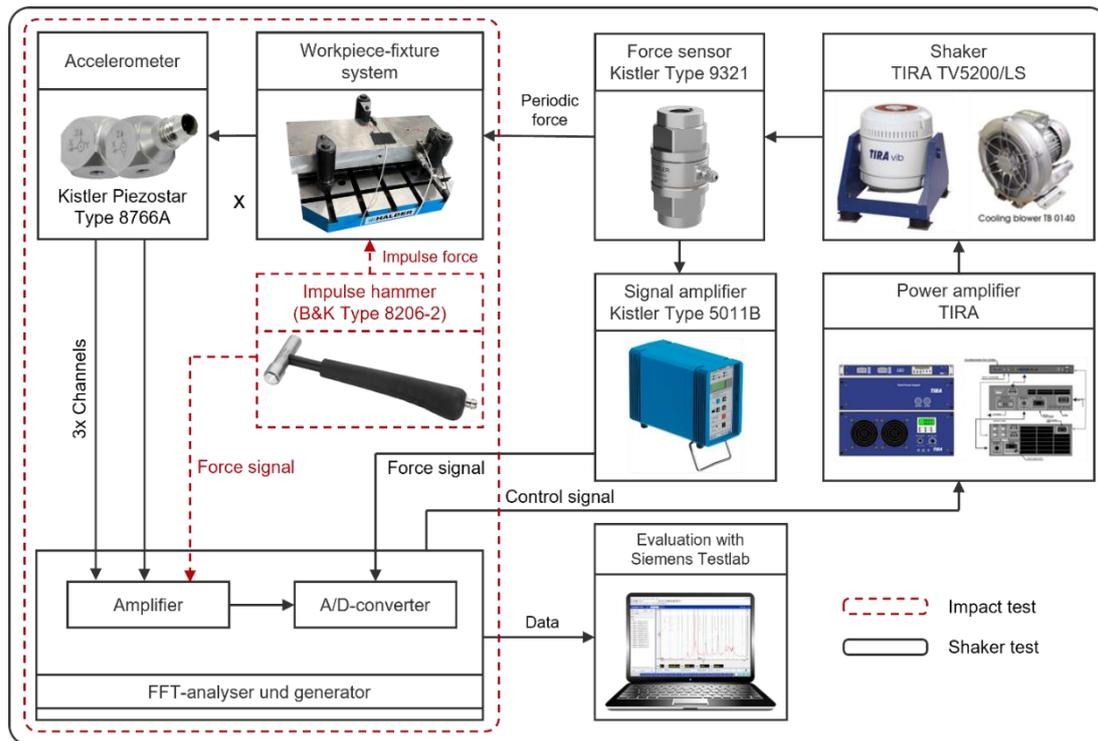
Fig. 3. Equipment for the experimental modal analysis: impact (circled in red) and shaker test (circled in black)
