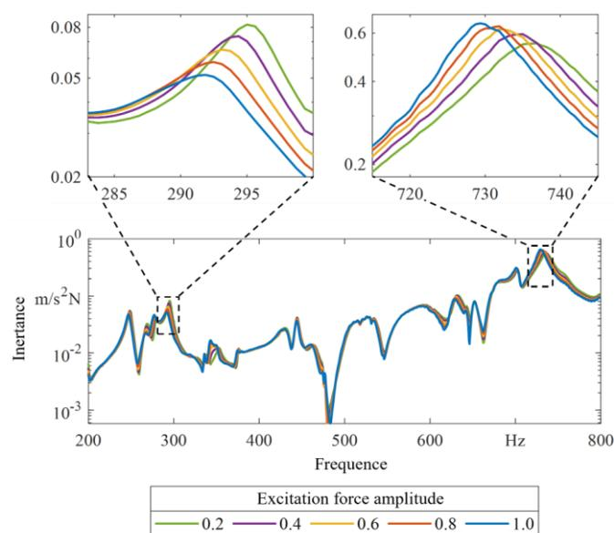
Fig. 6. Inertance for different excitation force amplitudes (excitation points 22/30, measuring point 28)
