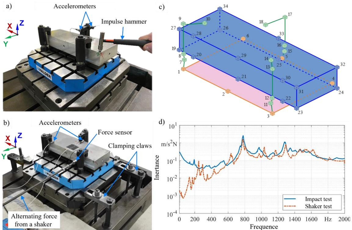
Fig. 4. a) Experimental setup of the impact test, b) setup of the shaker test, c) measuring points (1-34), excitation points (21/29 and 22/30 for the shaker test, 31 for the impact test), d) comparison of the frequency responses up to 2 kHz
