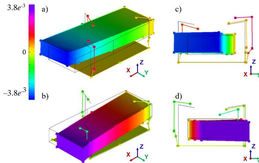
Fig. 5. Eigenmode at 295 Hz with 0.92% modal damping: displacement in  $\pm Y$  direction in the isometric view (a, b) and the side view (c, d), undeformed (black contour) and deformed (color)
