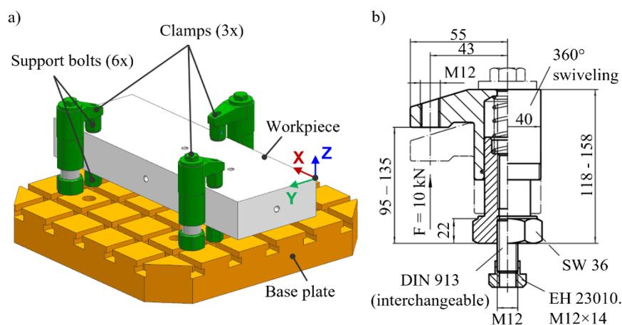
Fig. 2. a) Configuration of an exemplary workpiece-fixture system, b) dimensions of a down-thrust clamp
