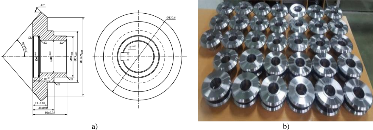
Fig. 1. Workpiece to manufacture the curved bevel gear: a) technical requirements of the workpiece, b) images of workpieces
