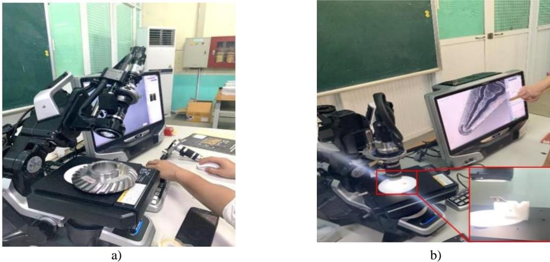
Fig. 3. Measurement of surface roughness and tool wear using a digital microscope (VHX600): a) measurement of surface roughness, b) measurement of tool wear
