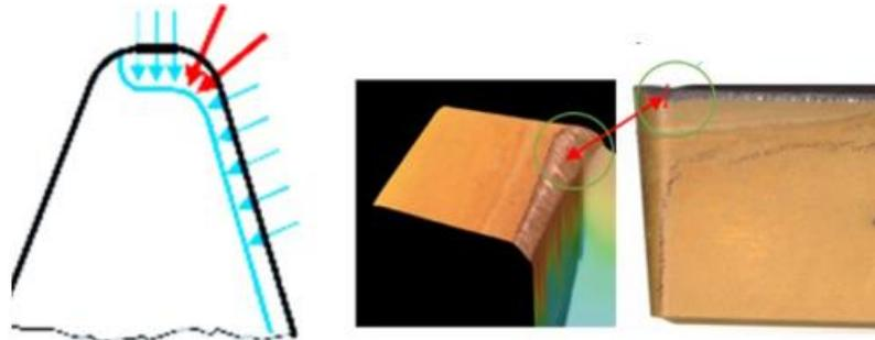
Fig. 5. Measurement position of tool wear
