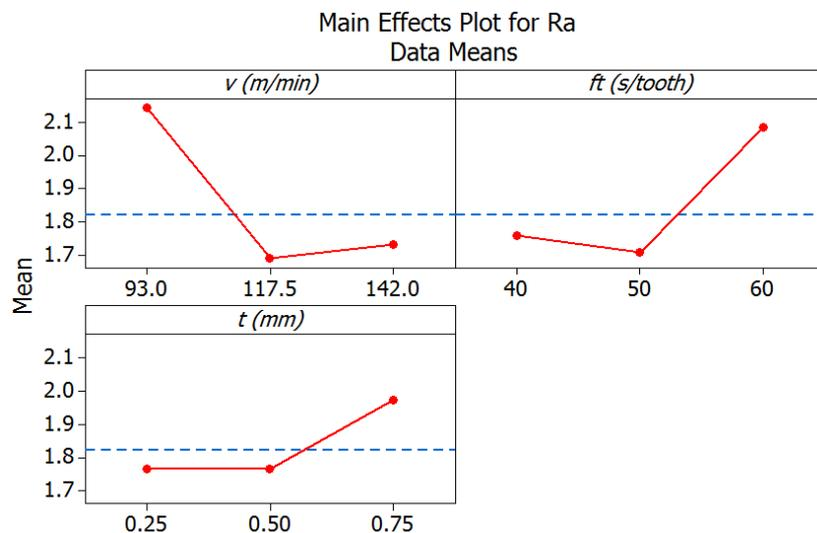
Fig. 6. Influence of cutting parameters on the surface roughness
