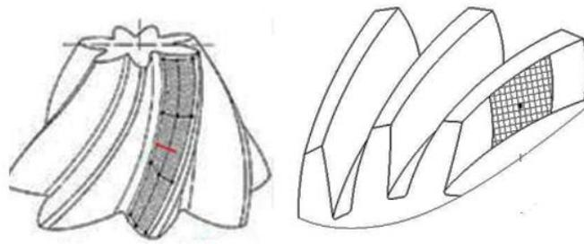
Fig. 4. Surface roughness measurement area (tooth flank)
