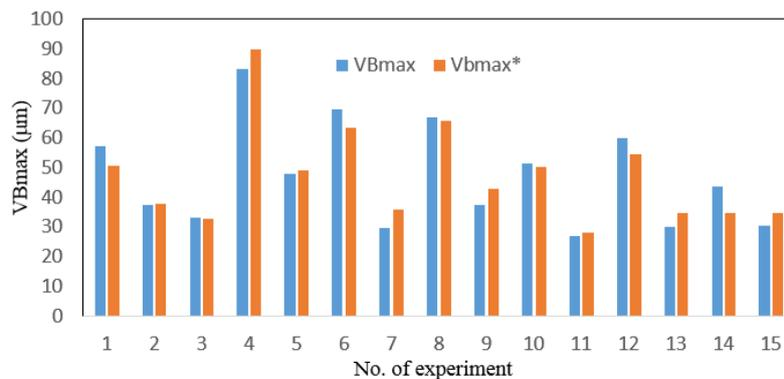
Fig. 9. Measured tool wear (VBmax) and predicted tool wear (VBmax\*)
