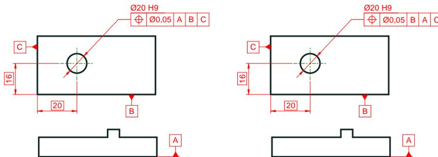
Fig. 10. Are these two specifications equivalent?
