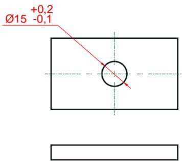
Fig. 8. Maximum material size for the hole is equal: ....
