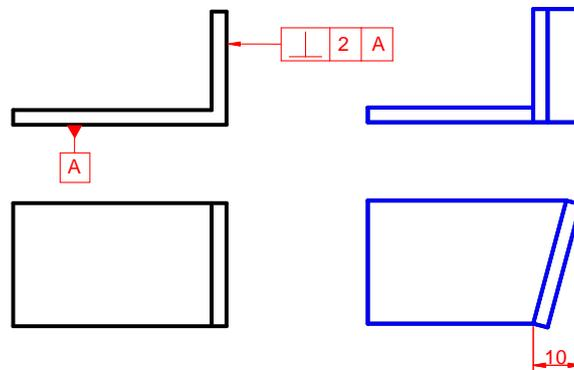
Fig. 4. After processing, the tilted top surface was observed. Does the product comply with the specification?
