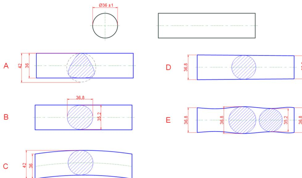
Fig. 1. After processing, a significant form deviation was observed. Which of the following products comply with the specification?
