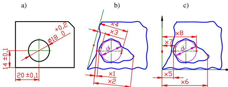
Fig. 6. a) Specification with  $\pm$  tolerancing; b), c). The ambiguity of specification with  $\pm$  tolerancing for an actual workpiece
