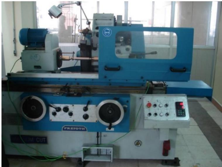
Fig. 1. External cylindrical grinding machine MEG–112
