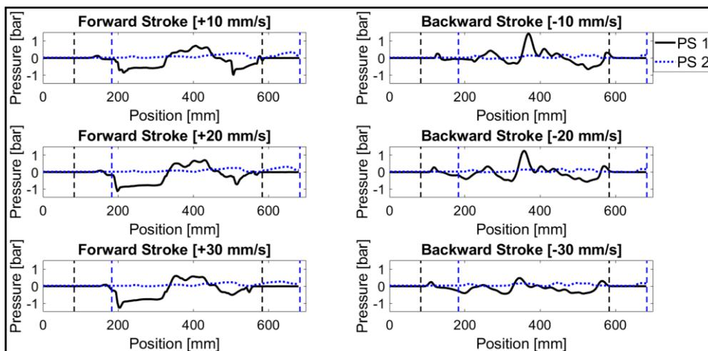
Fig. A2. The pressure measured for forward and backward strokes inside the lubrication gap using geometry variant I
