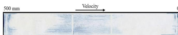
Fig. 9. Contact pattern developed between sliding bar and steel rail during sliding
