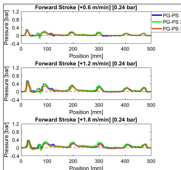
Fig. 2. Oil film pressure measured with sensors integrated in Plexiglas rail (shown in Fig. 1) with PG-PS-1, PG-PS-2 and PG-PS-3. Machine table with Surface pressure of 0.24 bar is considered in this case [13]
