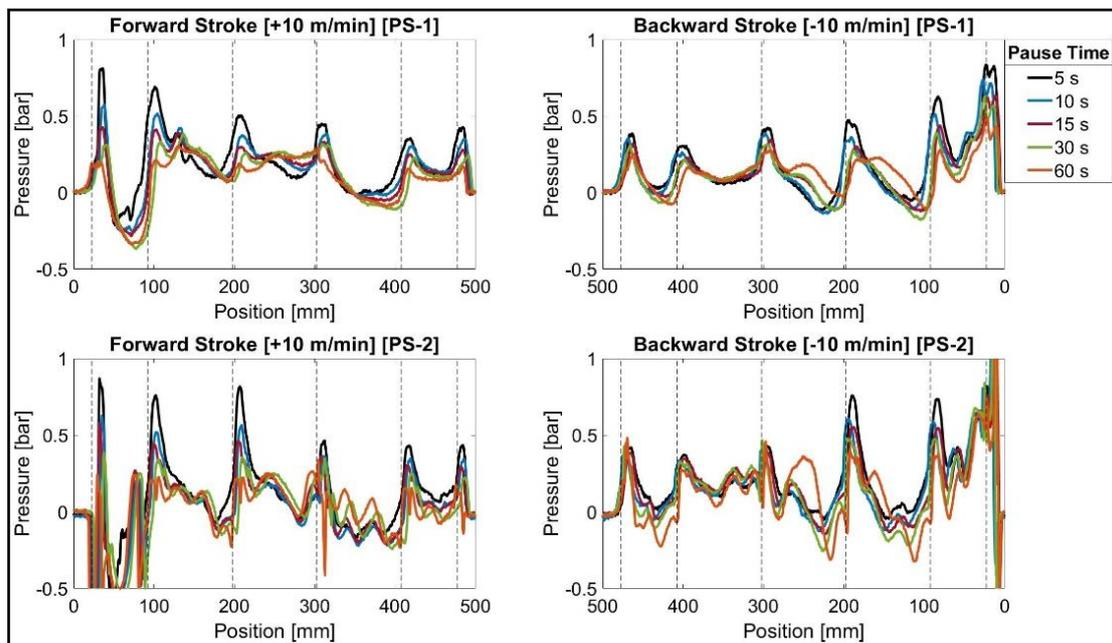
Fig. A4. The pressure peaks (6 peaks for 6 lubrication grooves) measured for forward and backward strokes inside the lubrication gap using geometry variant II for different pause time at 10 m/min
