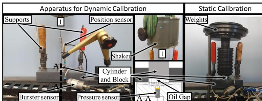
Fig. 3. Test-stand for both static calibration (Right) and dynamic calibration (Left) of sensors integrated in steel rail
