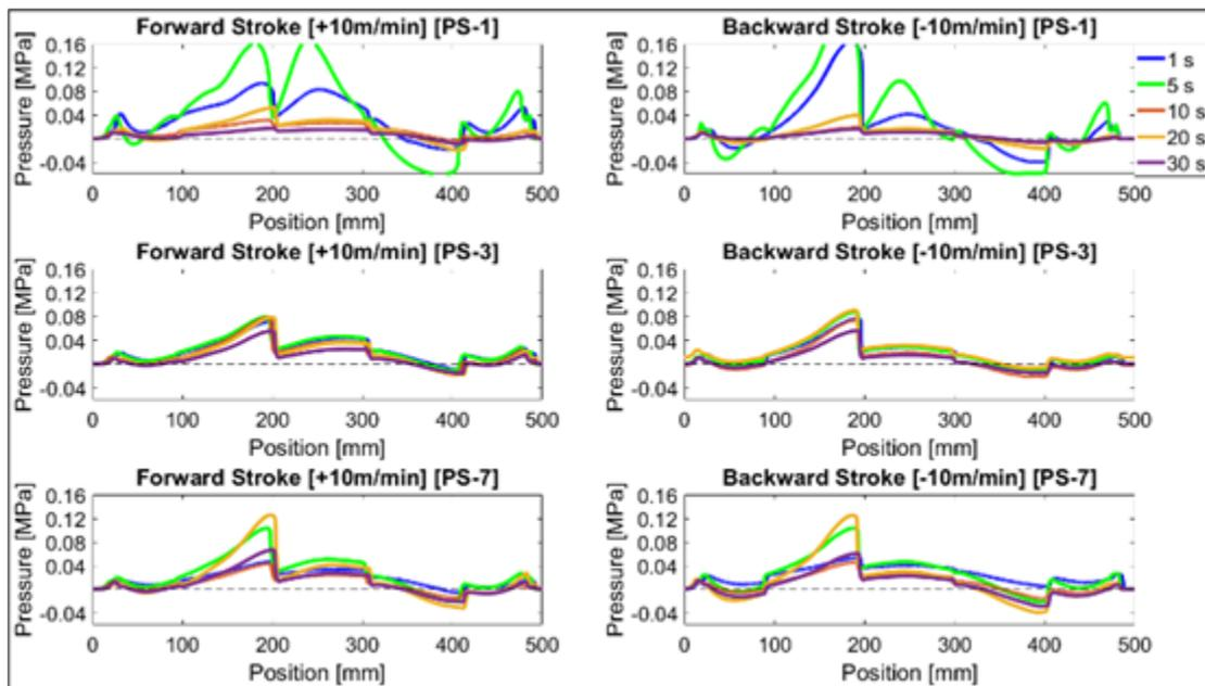
Fig. 14. Oil film pressure inside lubrication gap at different pause times for pressure sensors PS-1, PS-3 and PS-7 from top to bottom respectively. Left: Forward strokes and Right: Backward strokes, at 10 m/min feed-rate
