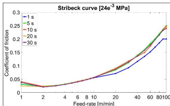
Fig. 15. Stribeck curve for different pause times at different feed-rates. Surface pressure of 0.24 bar is considered
