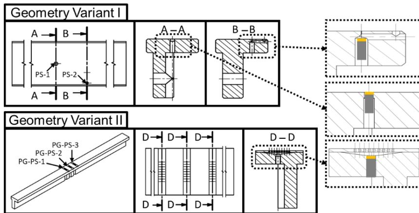
Fig. A1. Integration method of sensors for both geometry variants
