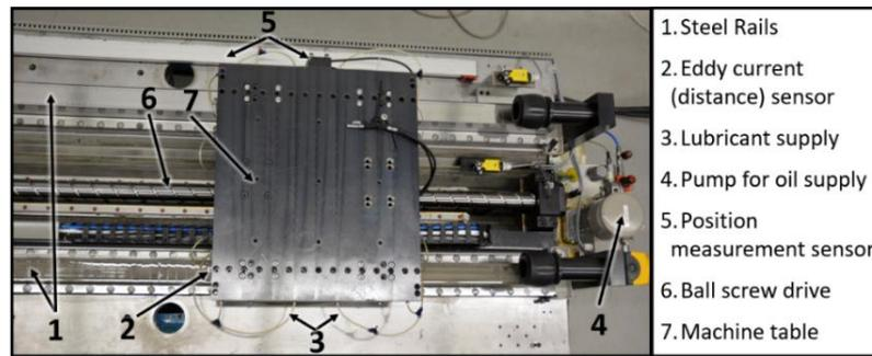
Fig. 6. Test-stand (Top-view) of hydrodynamic linear guides with pressure sensors integrated inside one steel rail
