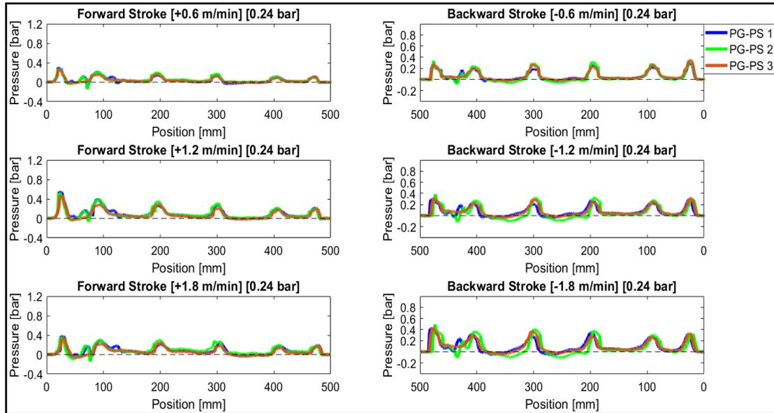
Fig. A3. The pressure peaks (6 peaks for 6 lubrication grooves) measured for forward and backward strokes inside the lubrication gap using geometry variant II
