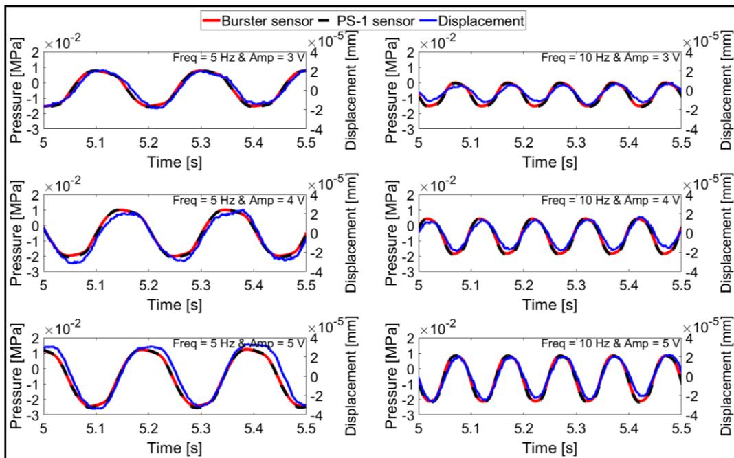
Fig. A6. Dynamic calibration of pressure sensor in steel rail and Burster sensor (for comparison) and displacement of cylinder (Experimental setup shown in Fig. A5)
