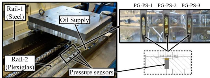
Fig. 1. Test-stand with Plexiglas rail and different integration methods of pressure sensors used by Ibrar [13]
