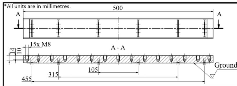
Fig. 8. Sketch of the sliding rails with 6 lubrication grooves
