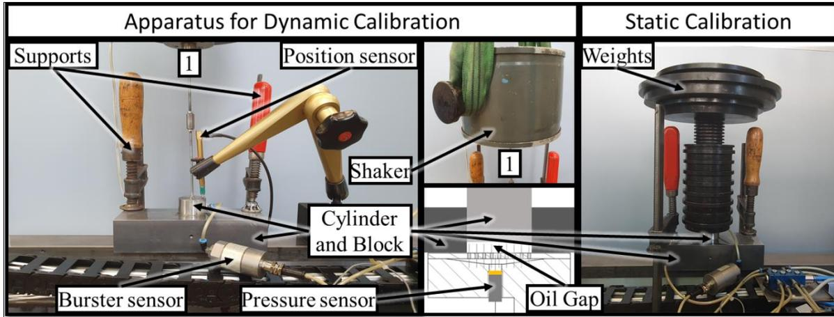
Fig. A5. Test stand for both static calibration (Right) and dynamic calibration (Left) of sensors integrated in steel rail
