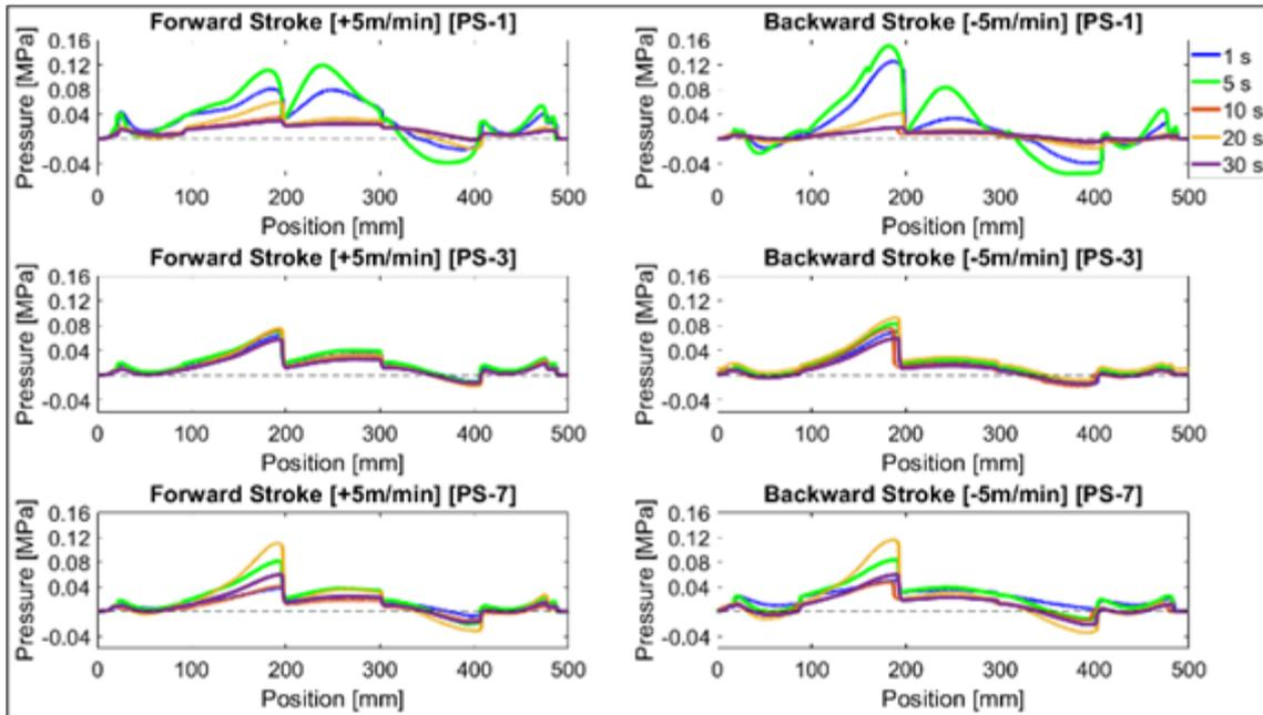
Fig. 13. Oil film pressure inside lubrication gap at different pause times for pressure sensors PS-1, PS-3 and PS-7 from top to bottom respectively. Left: Forward strokes and Right: Backward strokes, at 5 m/min feed-rate
