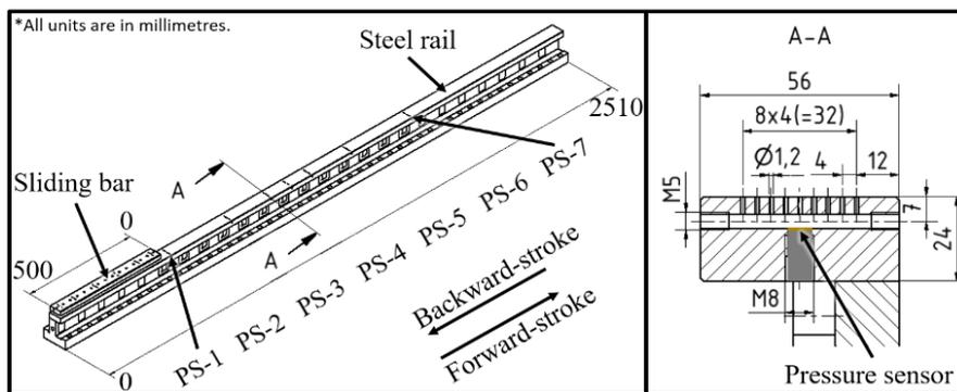
Fig. 7. Sketch of the steel-rail with integrated pressure sensors
