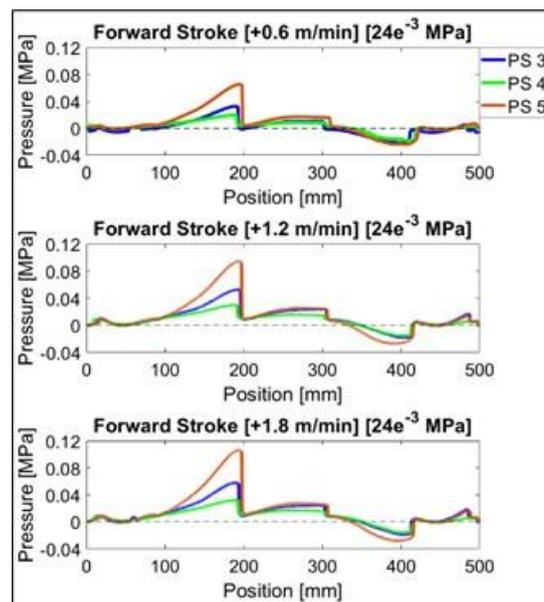
Fig. 10. Oil film pressure measured with sensors integrated in steel rail (shown in Fig. 7) with PS-3, PS-4 and PS-5. Machine table with Surface pressure of 0.24 bar is considered in this case
