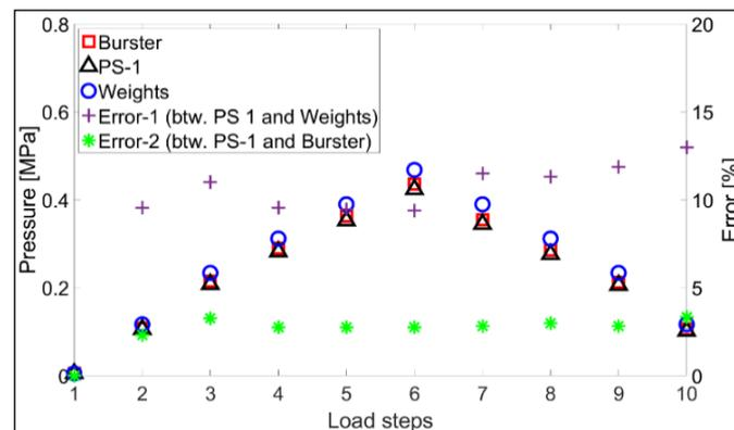
Fig. 4. Static calibration of pressure sensor in steel rail and comparison with Burster sensor and actual weights
