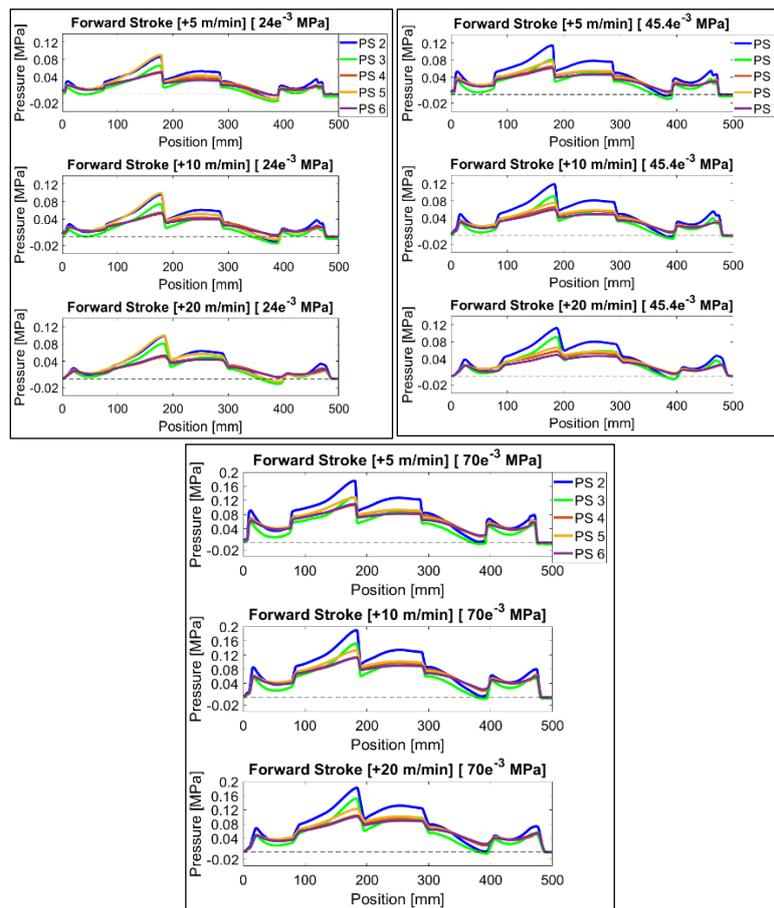
Fig. 11. Oil film pressure at different feed-rates (5, 10 and 20 m/min) with different pressure sensors (PS-2, PS-3, PS-4, PS-5, PS-6 and PS-7) integrated in a steel rail. Machine table with surface pressure of 0.24, 0.454 and 0.7 bar (Top-Left, Top-Right and Bottom respectively) is considered in this case
