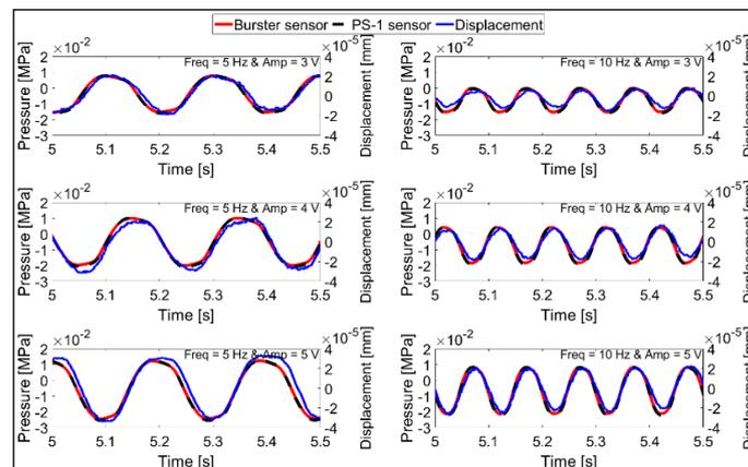
Fig. 5. Dynamic calibration of pressure sensor in steel rail and Burster sensor (for comparison) and displacement of cylinder
