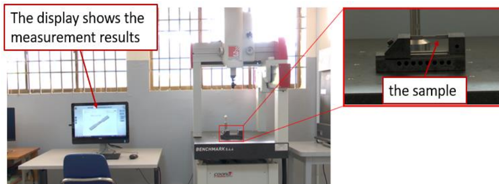
Fig. 6. Measure the size and geometry of the sample
