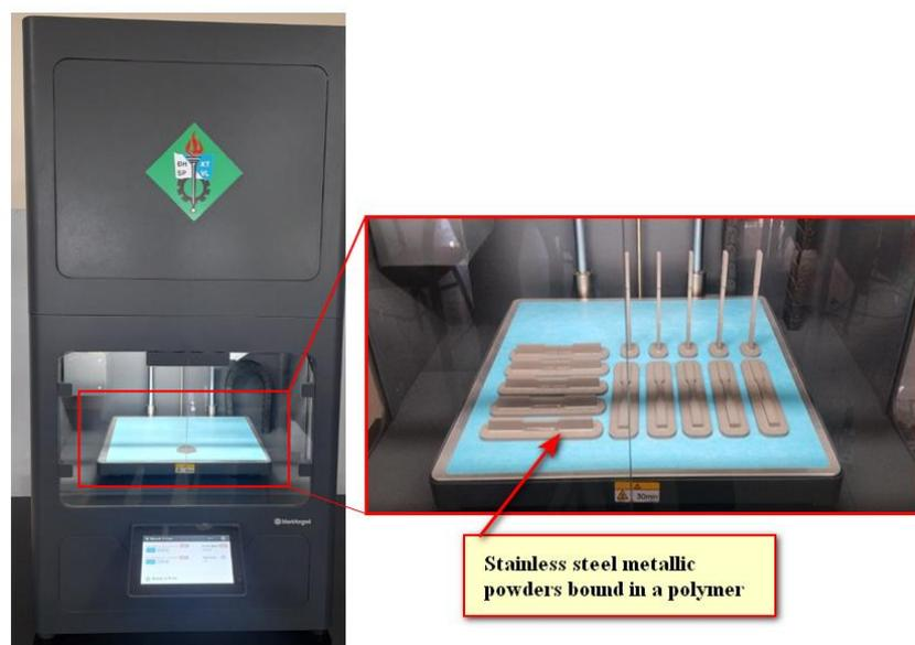
Fig. 3. Experiments on the ME machine
