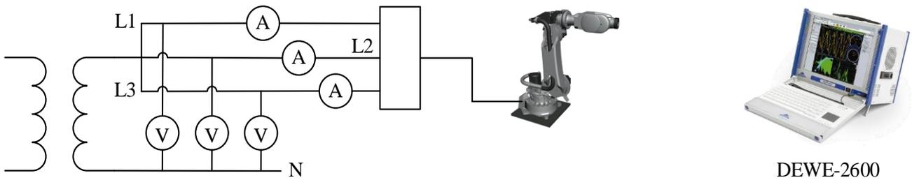
Fig. 4. Structural measurement setup and measured variables
