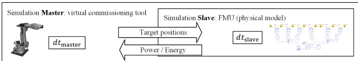
Fig. 8. Master-slave arrangement in the Co-Simulation and exchanged variables
