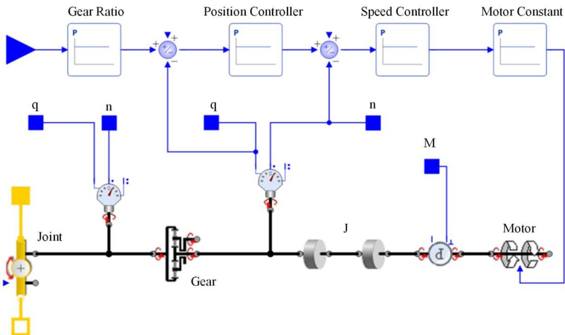
Fig. 3. Drive module with control loops, inertias, gear and joint
