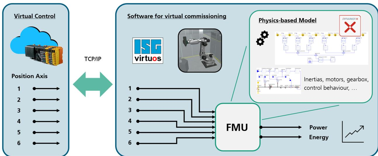
Fig. 7. Structural design of the SiL simulation in the virtual commissioning environment
