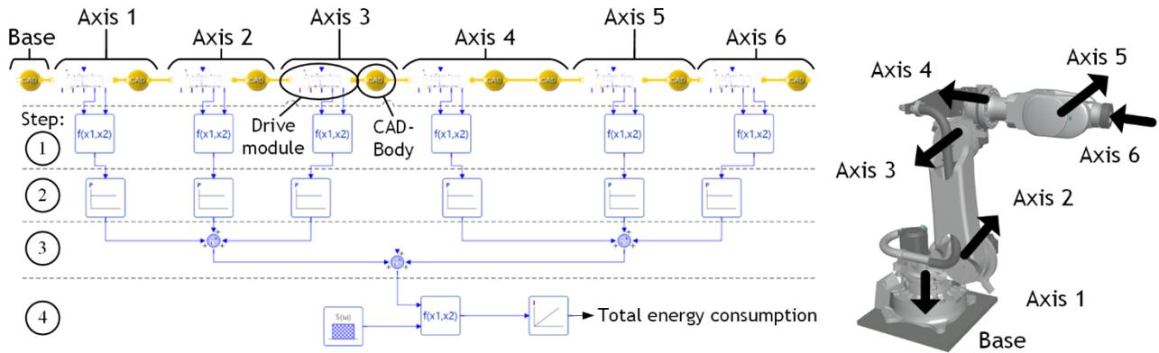
Fig. 2. Physical model of the 6-axis Comau robot modelled in SimulationX
