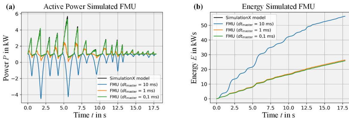
Fig. 9. FMU results for different simulation step sizes of simulation master: (a) power curve, (b) energy consumption
