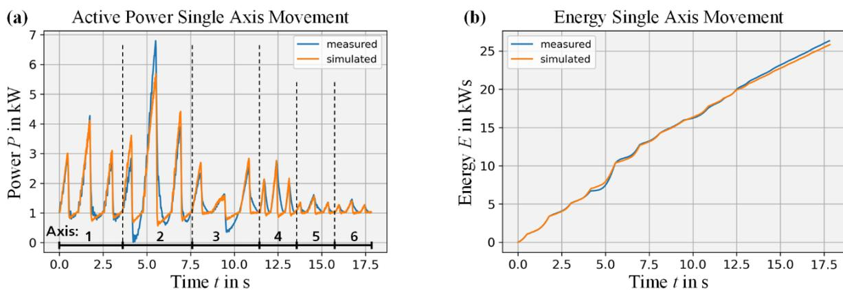
Fig. 6. Comparison of measurement and simulation for the aligned model: (a) power curve, (b) energy consumption
