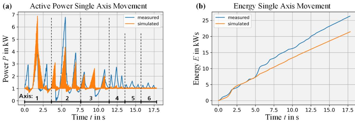
Fig. 5. Comparison of measurement and simulation for robot movement: (a) power curve, (b) energy consumption
