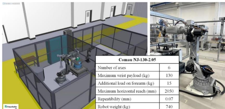
Fig. 1. Robot cell used as application example
