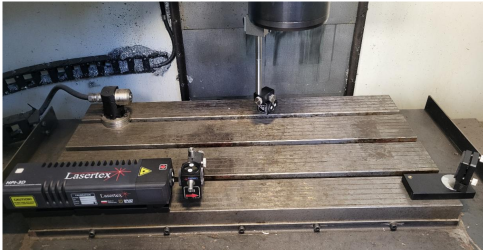
Fig. 8. Placement of device components on the tested machine
