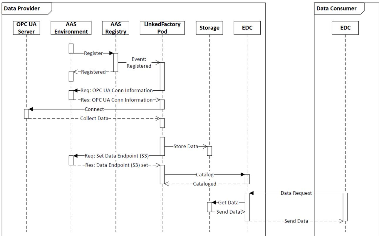
Fig. 8. Sequence diagram of the proposed data pipeline
