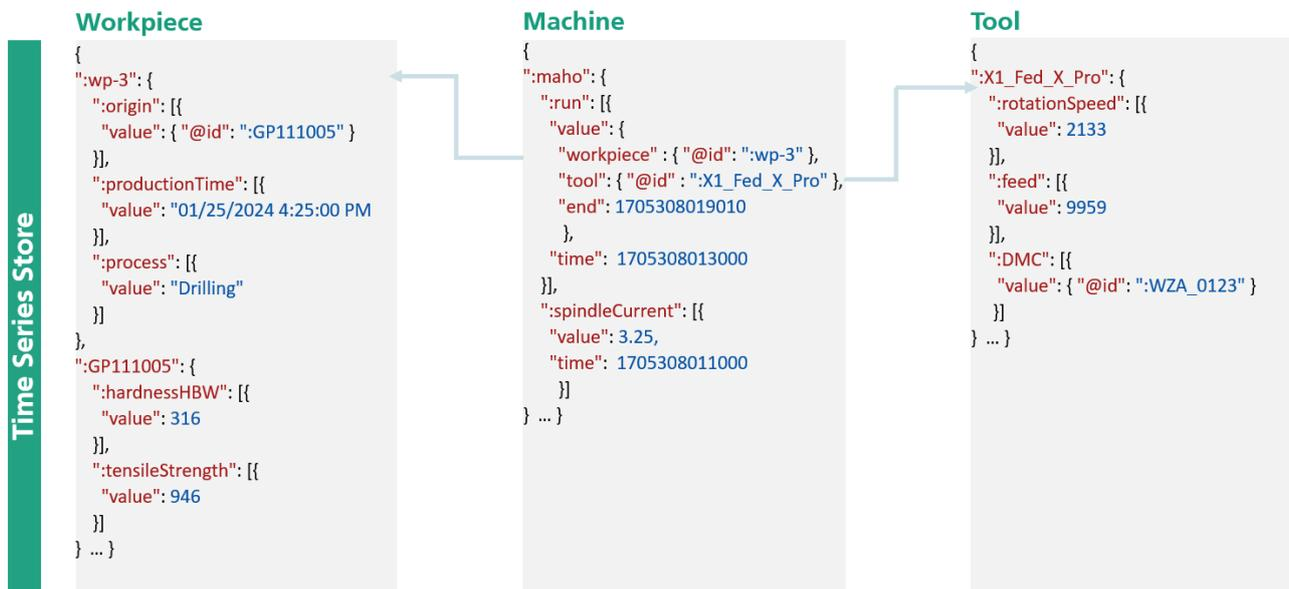
Fig. 7. Connection of different time series items for machine, workpiece and tool (data linking)
