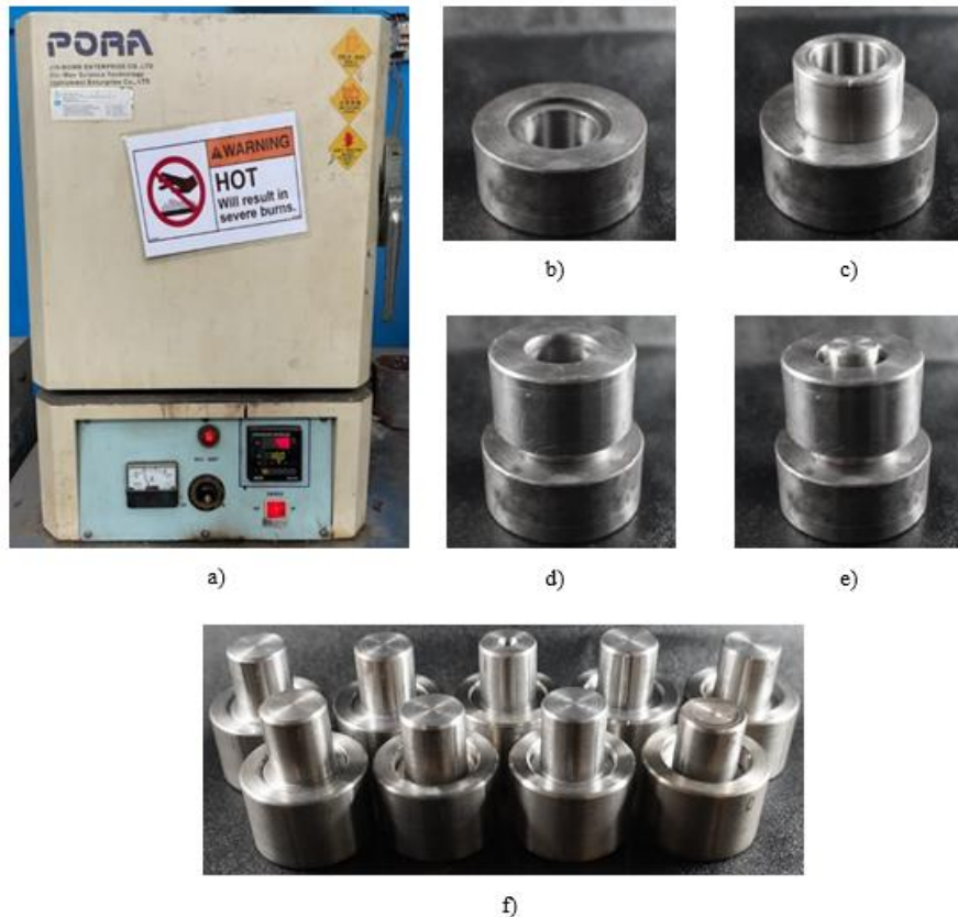
Fig. 2. Shrink-fitting process (SF process) and equipment
