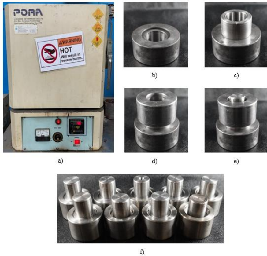
Fig. 2. Shrink-fitting process (SF process) and equipment
