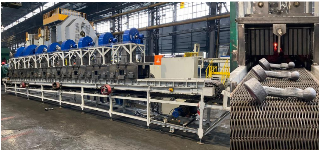
Fig. 6. Conveyor and products leaving controlled cooling
