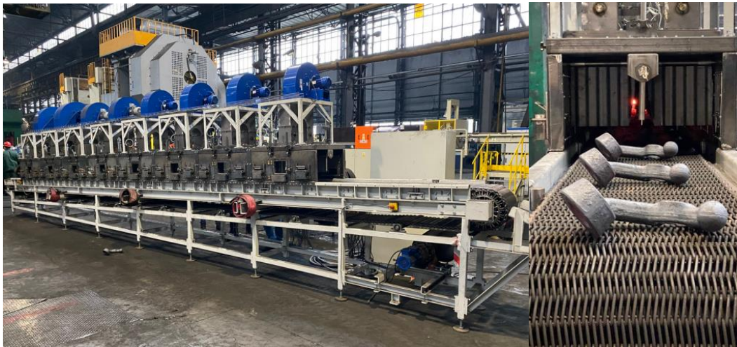
Fig. 6. Conveyor and products leaving controlled cooling
