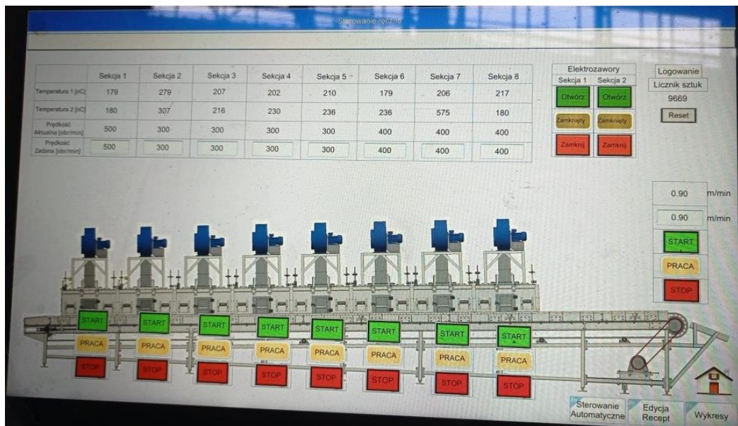
Fig. 7. Conveyor operation controller screen
