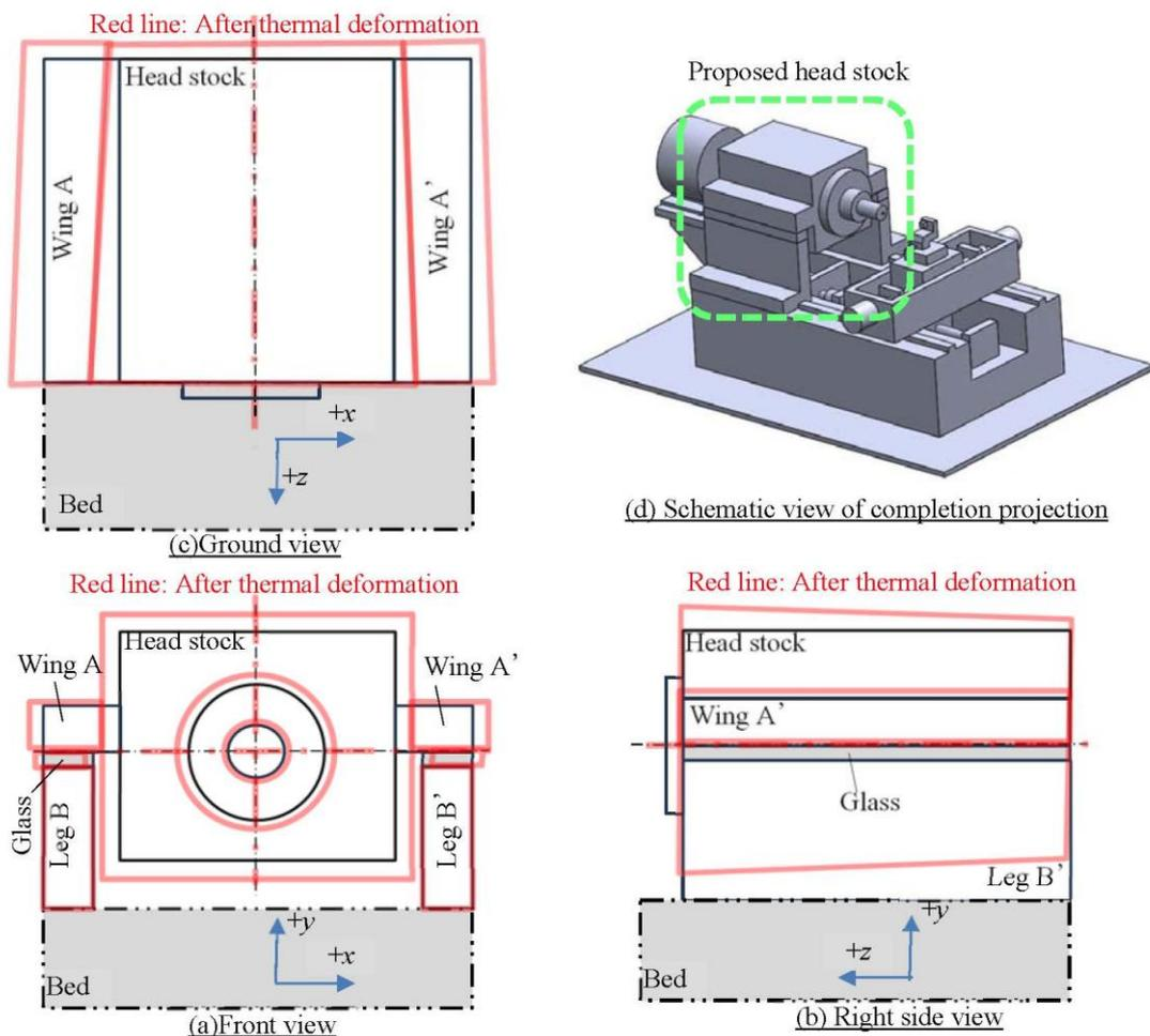
Fig. 2. Schematic view of the thermally insensitive structure for x-axis, y-axis, A-axis and B-axis directions on the head stock. Thermally insensitive structure of the two internal heat sources (front bearing and rear bearing) to thermal deformation
