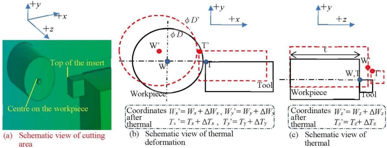
Fig. 1. Calculation method for the machining accuracy using the analysis results of FEM static simulation
