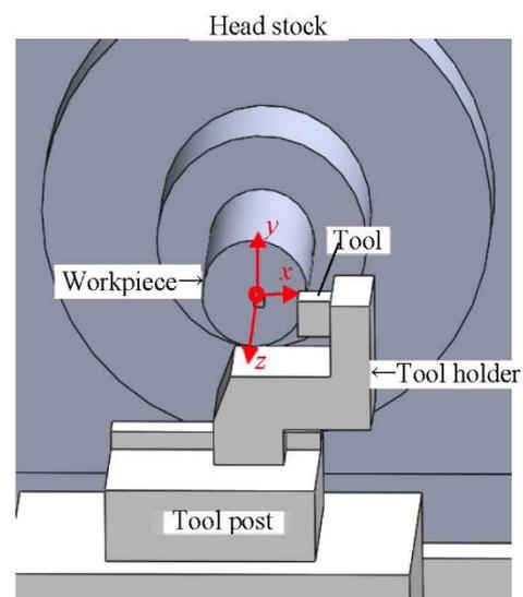
Fig. 4. The tool post is driven in the  $x=0$ ,  $y$ - $z$  plane (directly below the workpiece) for infeed movements. To make the cut from the  $x$ -axis direction, an odd-shaped toolholder is used
