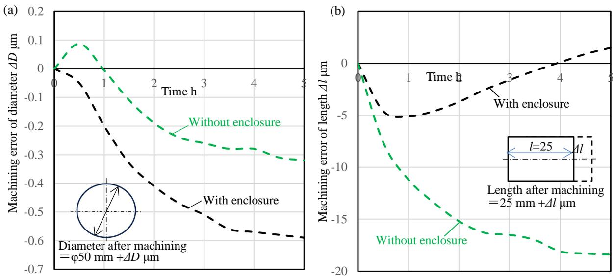
Fig. 12. Machining errors for 5 hours on the bench lathe with thermally insensitive structure, (a) – Machining error of diameter on the workpiece, (b) – Machining error of length on the workpiece
