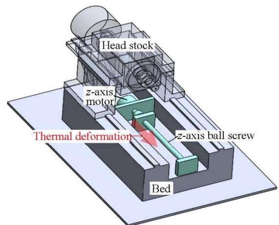
Fig. 6. The starting point for thermal deformation of the  $z$ -axis driving system is located directly below the workpiece in the cutting area
