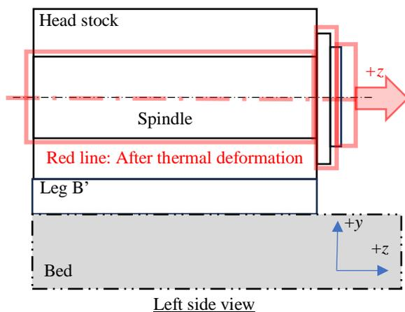
Fig. 5. The head stock is thermally deformed by the heat generated by the front and rear bearings, which thermally deforms the spindle in the  $+z$  direction
