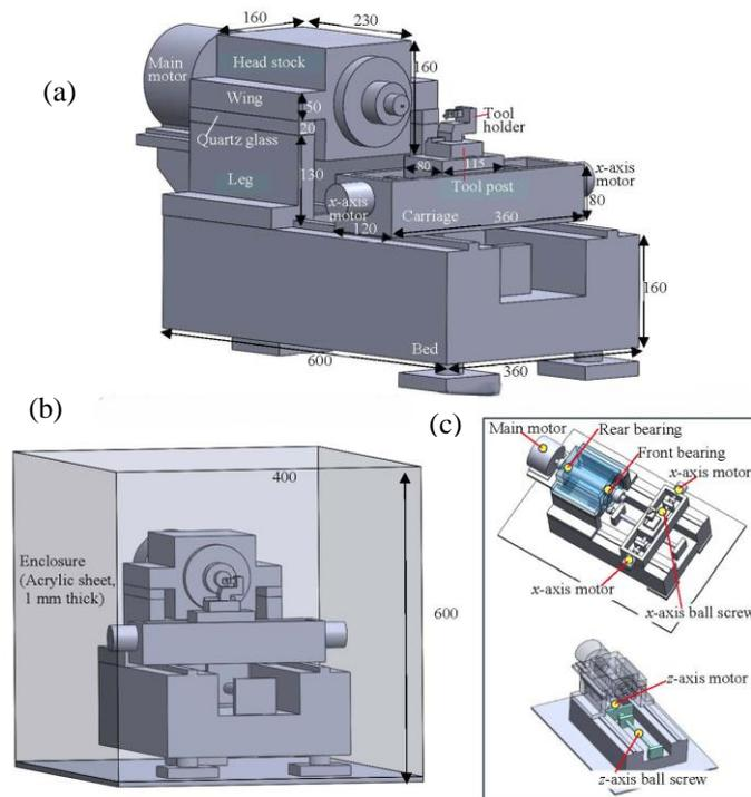
Fig. 7. Schematic view of the bench lathe with thermally insensitive structure (Enclosure hidden) – (a), Schematic view of the bench lathe with enclosure (Bench lathe hidden) – (b), Inner heat source positions – (c)
