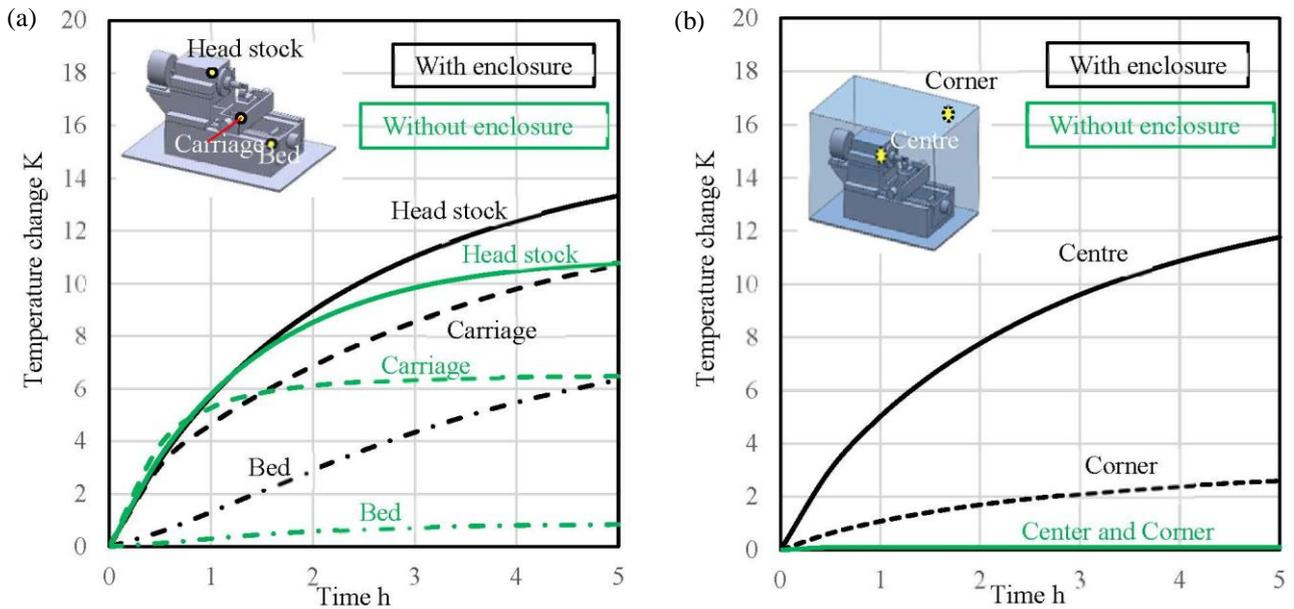
Fig. 9. Temperature distribution change on the machine structure – (a), Temperature distribution change on the atmosphere in the enclosure – (b)
