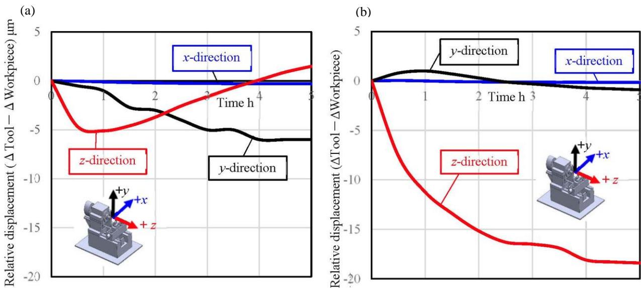
Fig. 10. Relative and thermal displacement changes for 5 hours on the bench lathe with thermally insensitive structure: (a) – With enclosure, (b) – Without enclosure
