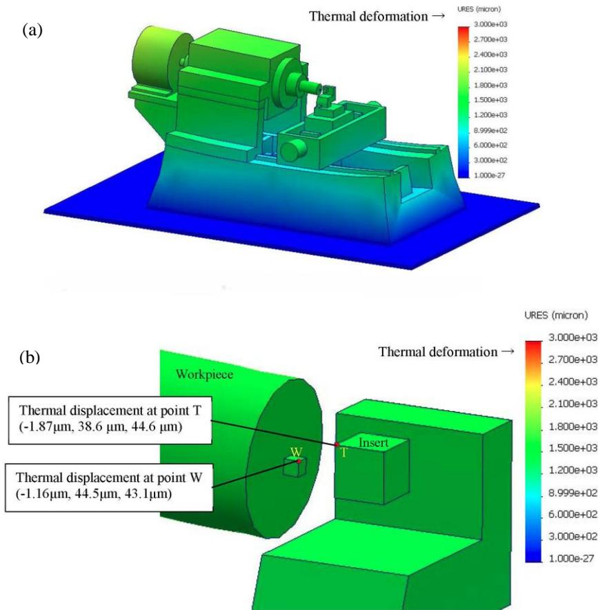
Fig. 11. An example of an FEM simulation regarding the thermal deformation on the bench lathe with thermally insensitive structure, (a) – Schematic view of thermal deformation on the bench lathe with enclosure, (b) – Around the cut ting area, (Enclosure hidden, Condition: Fig. 10 (a), at 5 hours)
