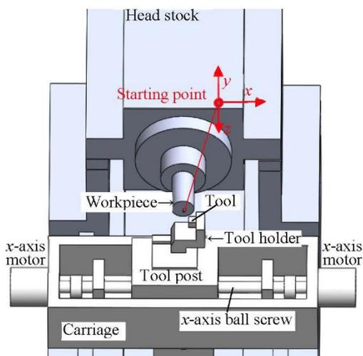
Fig. 3. Schematic view of the thermally insensitive structure for  $x$ -axis direction on the tool post and the carriage. The tool post and the carriage are symmetrically located in the  $x=0$ ,  $y$ - $z$  plane. Therefore, the  $x$ -axis driving system was used twin motors
