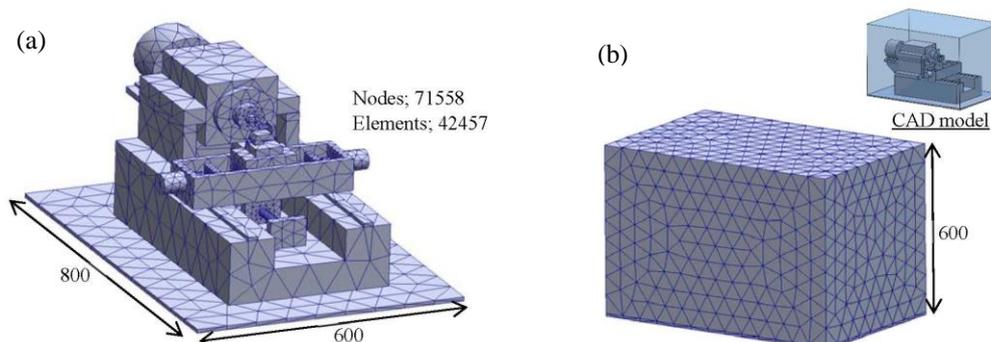
Fig. 8. FEM model with meshing for the heat insensitive structure bench lathe (Enclosure hidden) – (a), FEM model with meshing for the enclosure – (b)
