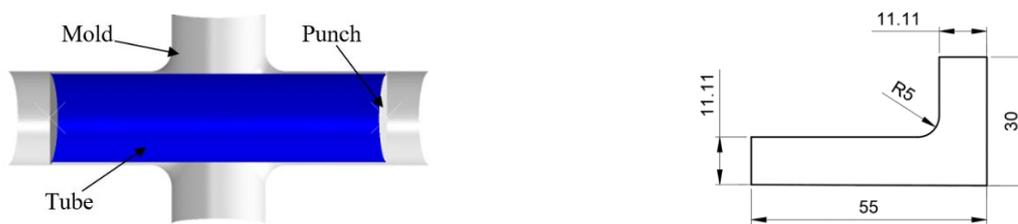
Fig. 3. Basic specifications of the die
