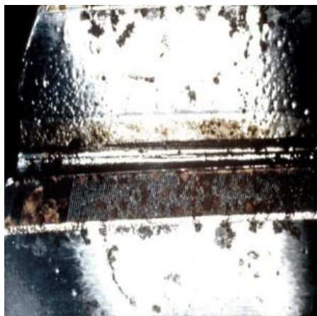
Fig. 6. Corrosive damage to tooth surfaces [3]
