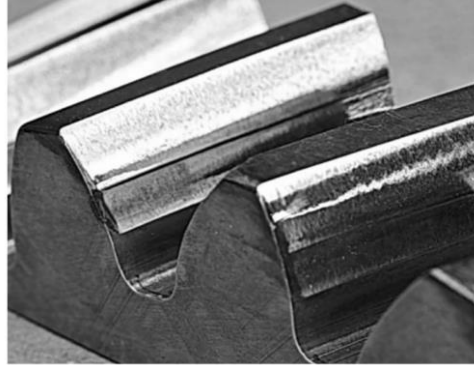
Fig. 5. Traces of adhesive wear in form of scuffing on surface of tooth roots and tips [7]
