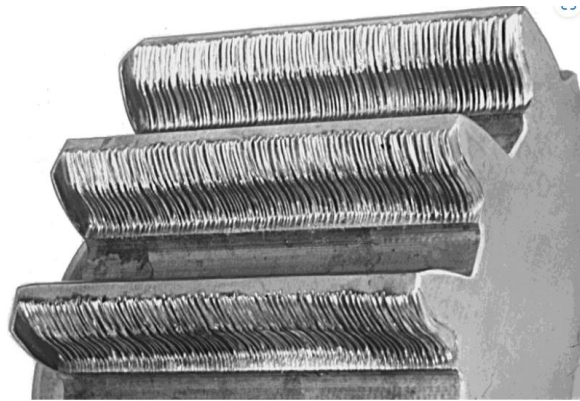
Fig. 3. Traces of excessive wear in form of grooves in gear wheel surface [7]
