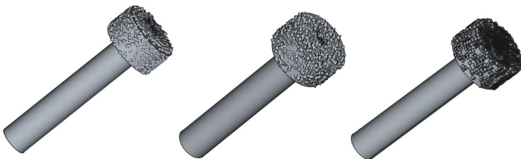
Fig. 4. Exemplary CAD models of grinding pins with diamond grains obtained in the FreeCAD software on the basis of Python code created in the ChatGPT™ represented by spheres, cones and cuboids
