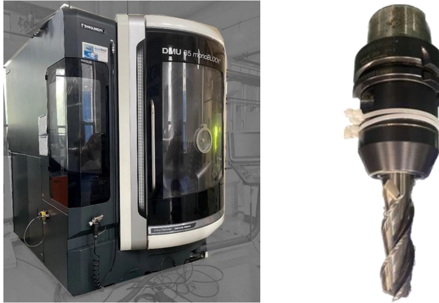
Fig. 3. DMG MORI DMU 65 monoBLOCK (left). „Unbalance” anomaly induced by adding a mass on one side of the spindle, causing an unbalanced spindle (right). Even though the mass added is small, the deviations are noticeable in the signals
