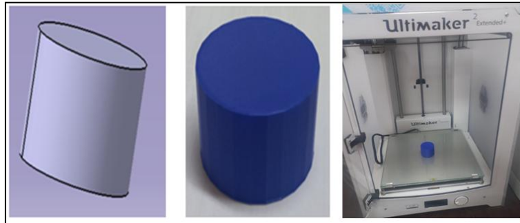
Fig. 6. Test part manufactured and FDM machine Ultimaker used
