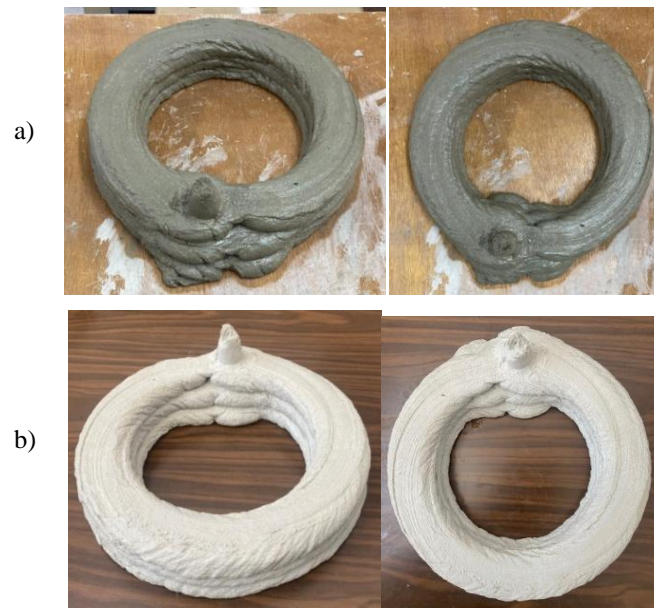
Fig. 13. (a) The printed circular wall after 1 hour and (b) after 28 days
