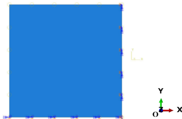
Fig. 3. Boundary conditions set for the springback simulation
