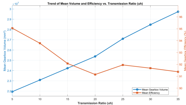
Fig. 3. Mean trends of gearbox volume and efficiency as functions of u_h
