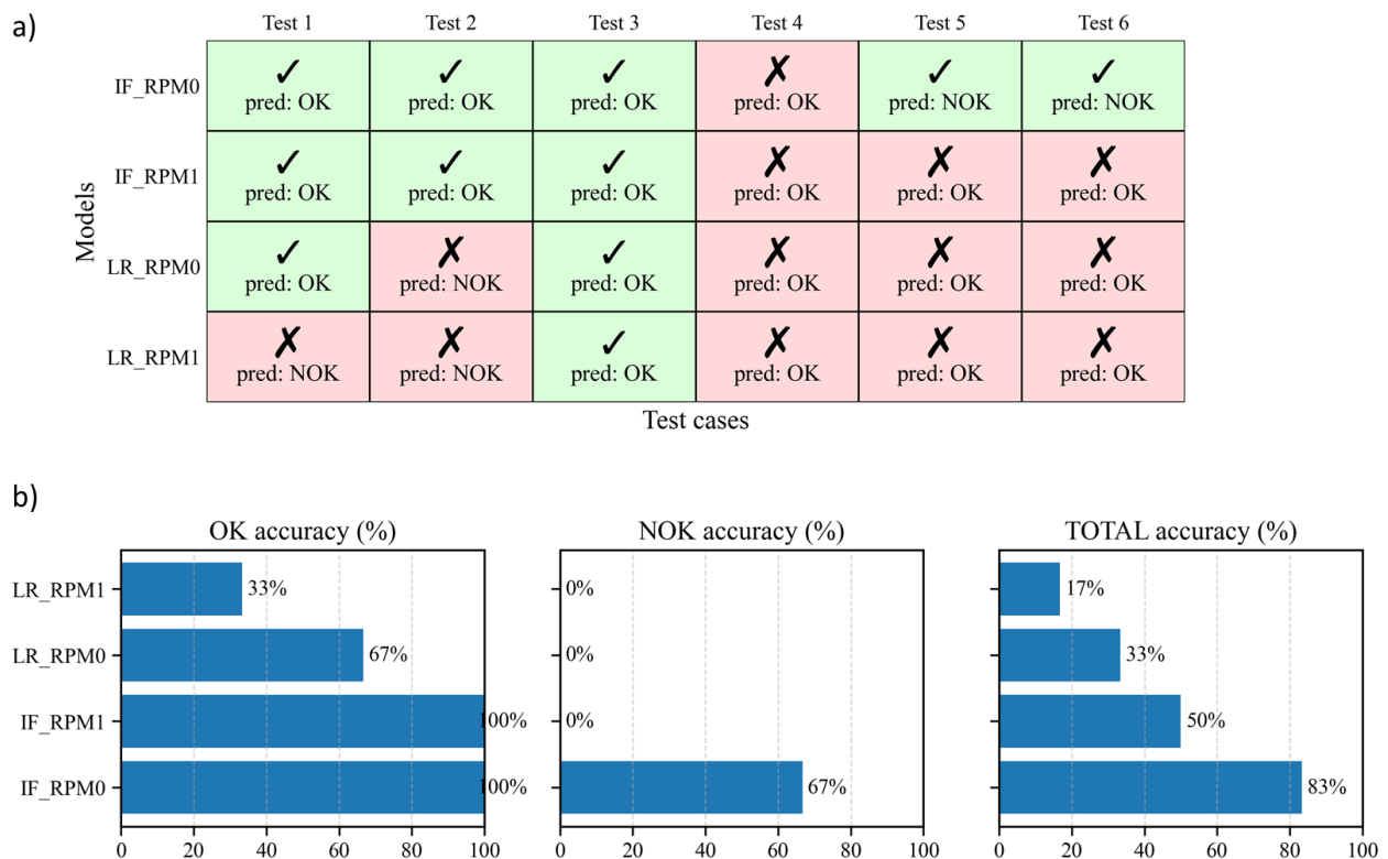
Fig.6. Deployment results on six unseen gearbox test cases. a) Prediction correctness matrix for Isolation Forest (IF) and Logistic Regression (LR) models for RPM0 and RPM1. b) Comparison of OK-class accuracy, NOK-class accuracy, and overall accuracy across models
