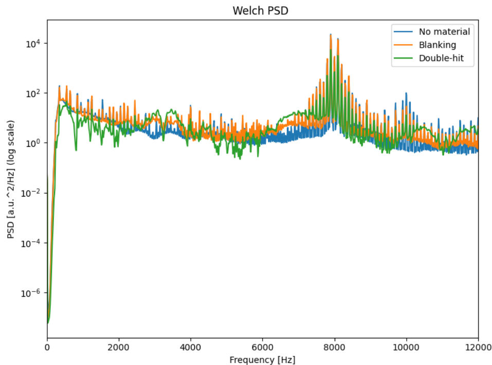
Fig. 5. Averaged power spectral density (PSD) spectra of vibroacoustic signals recorded under no-material, normal blanking (0.5 mm CuZn37), and simulated double-hit (0.1 mm spacer) conditions
