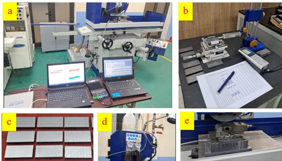
Fig 1. Schematic of the experimental setup: a) Overview of the surface grinding system, b) Surface roughness measurement; c) Workpiece samples, d) MQL supply system, e) Kistler dynamometer setup
