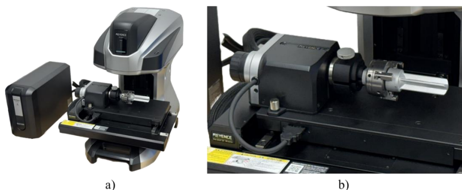
Fig. 5. Keyence VR6000 (a) and 360° scanning setup using the rotational module (b)
