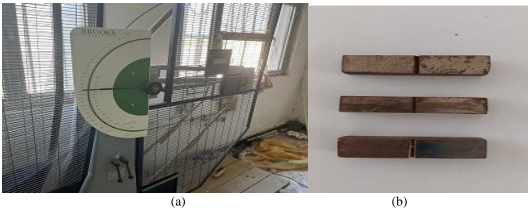
Fig. 6. (a) A BROOKS Charpy Impact Testing Machine, (b) Impact sample of charpy test
