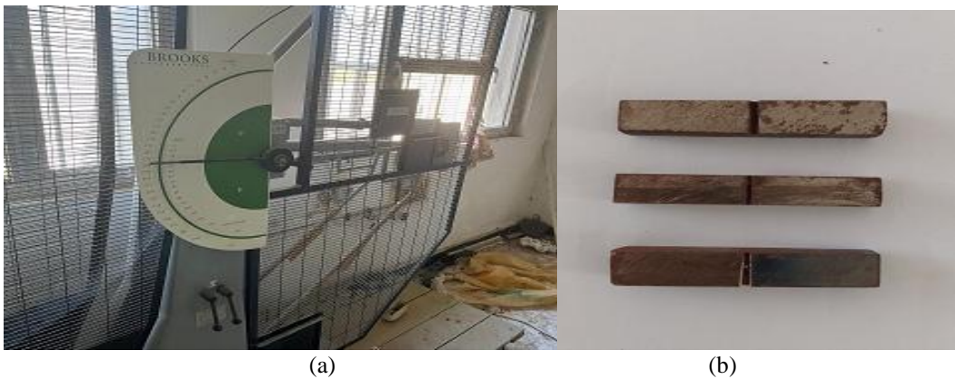
Fig. 6. (a) A BROOKS Charpy Impact Testing Machine, (b) Impact sample of charpy test
