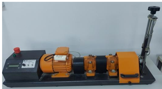
Fig. 5. Fatigue testing device used in the current study
