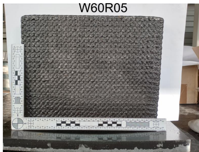
Fig. 3. Wall after printing–W60R05
