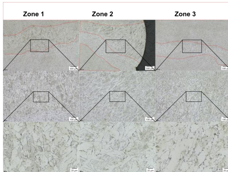
Fig. 21. Microstructure variation over different zones
